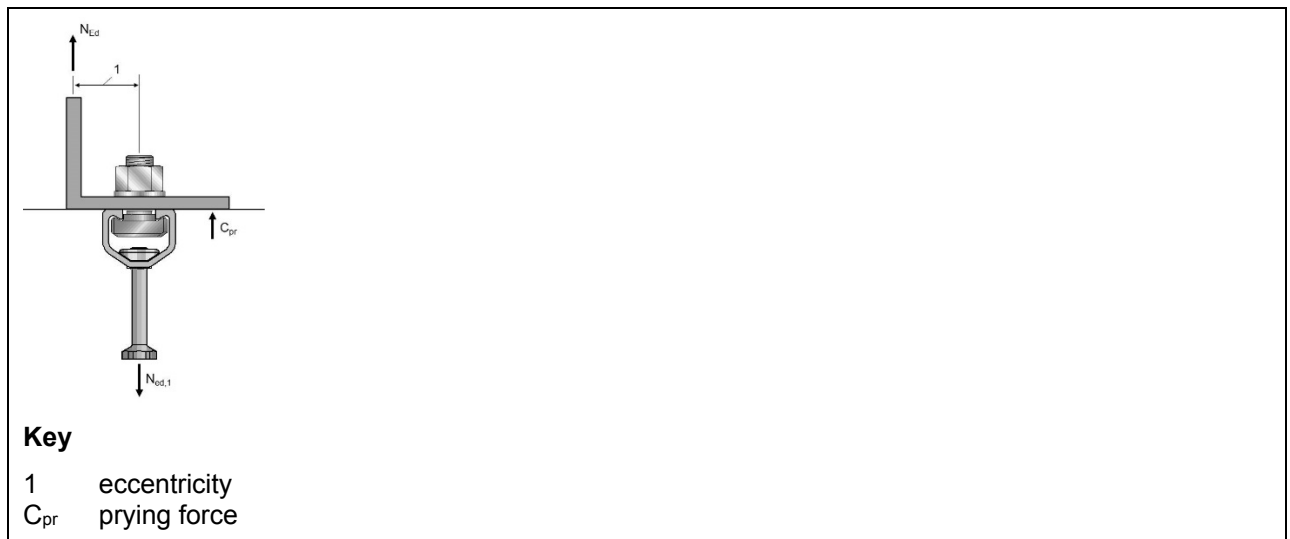
Figure 6.1 Examples for amplification of tension forces acting on the anchor channel due to eccentricity
