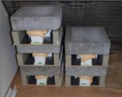
Figure 5: Test sample during curing (48hrs)
