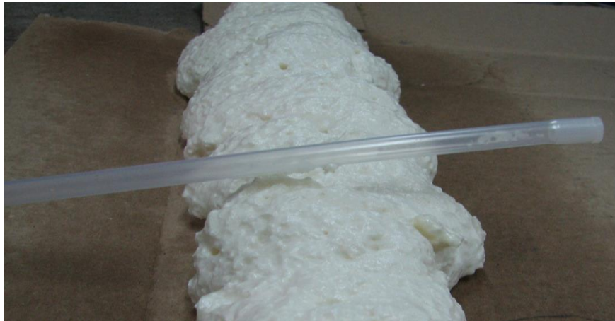
Figure 1 – Touching the bead with the rod/tube
