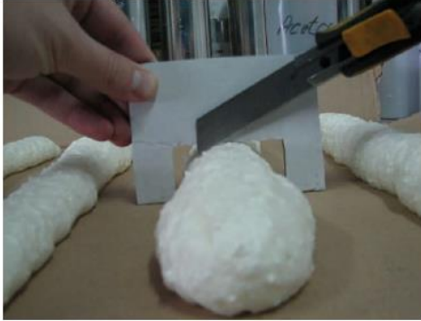
Figure 3: How to find 3 cm diameter bead
