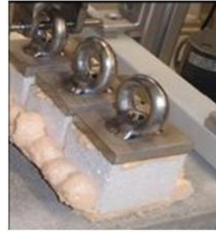
Figure F.4.6: Tie anchors
