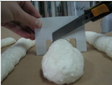
Figure 3: How to find 3 cm diameter bead
