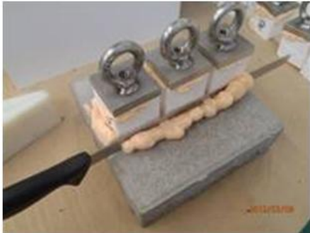
Figure F.4.7: Cutting of the surplus
