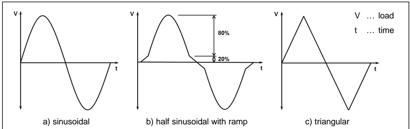
Figure E.9 Permitted seismic shear cycle C1.2
