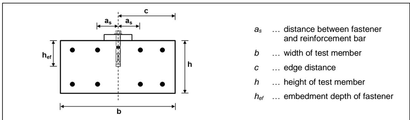
Figure E.1 Example cross section of test member
