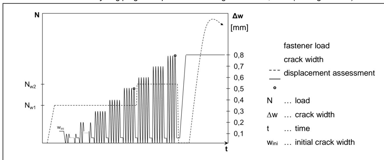
Figure E.13 Schematic test procedure C2.5
