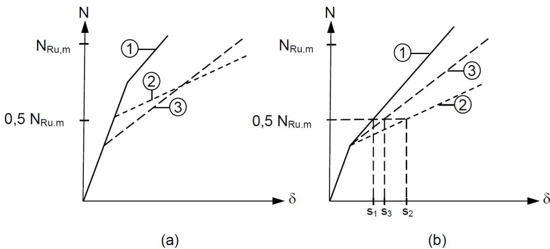
Figure A.6 Influence of pre-stressing on load/displacement curves
