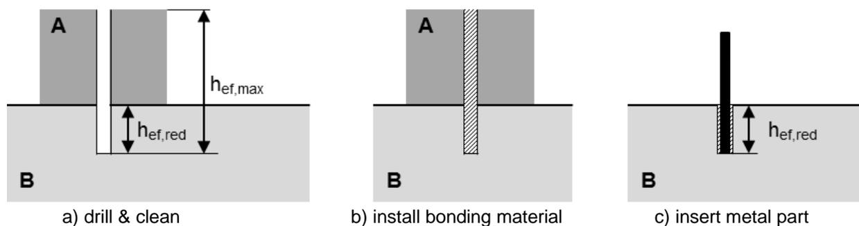
Figure A.1 Test set up to avoid steel failure
