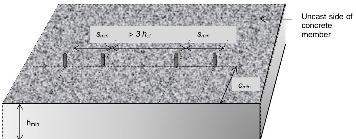
Figure 2.2 Installation of fasteners at the edge of concrete member
