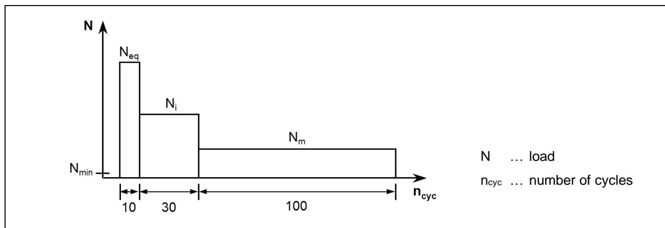
Figure E.7 Required loading history for test series C1.1
