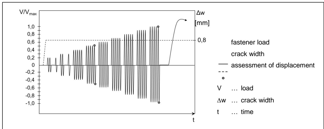
Figure E.11 Schematic test procedure C2.4
