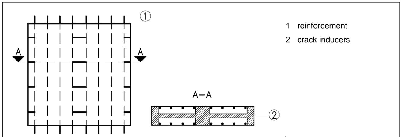
Figure D.2 Example of a test member for fasteners tested in cracked concrete
