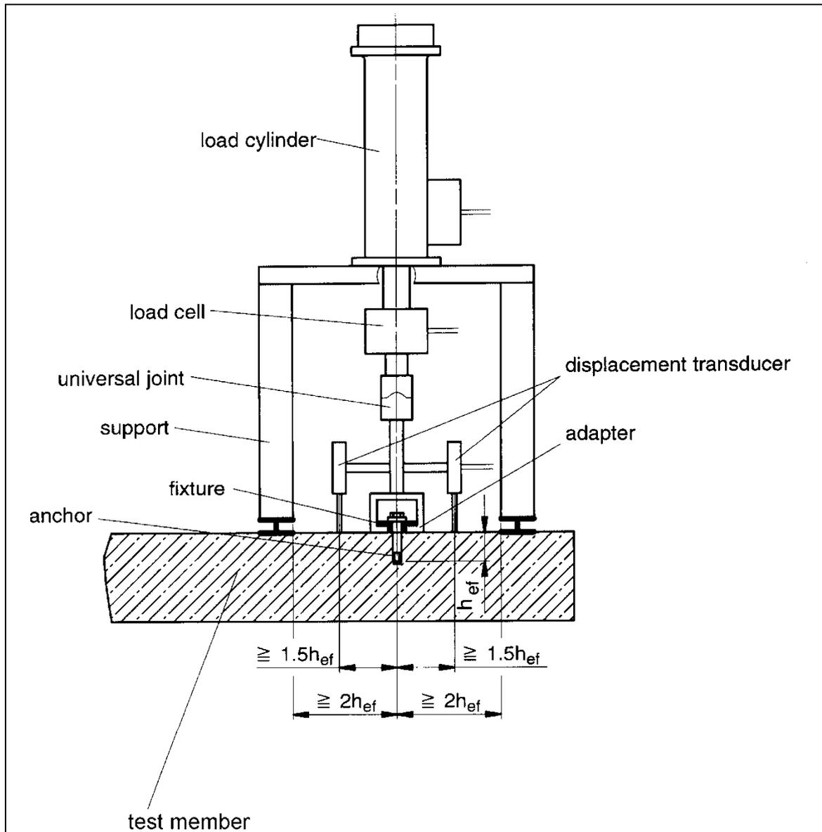
Figure D.3 Example of a tension test rig for unconfined tests
