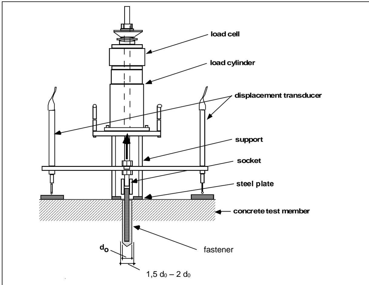
Figure D.4 Example of a tension test rig for confined tests
