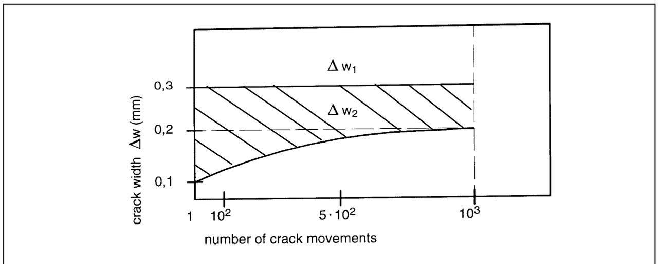
**Figure D.11 Allowable crack opening variations during the crack movement test**
