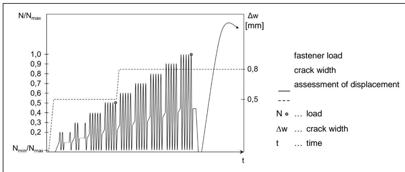
Figure E.10 Schematic test procedure C2.3
