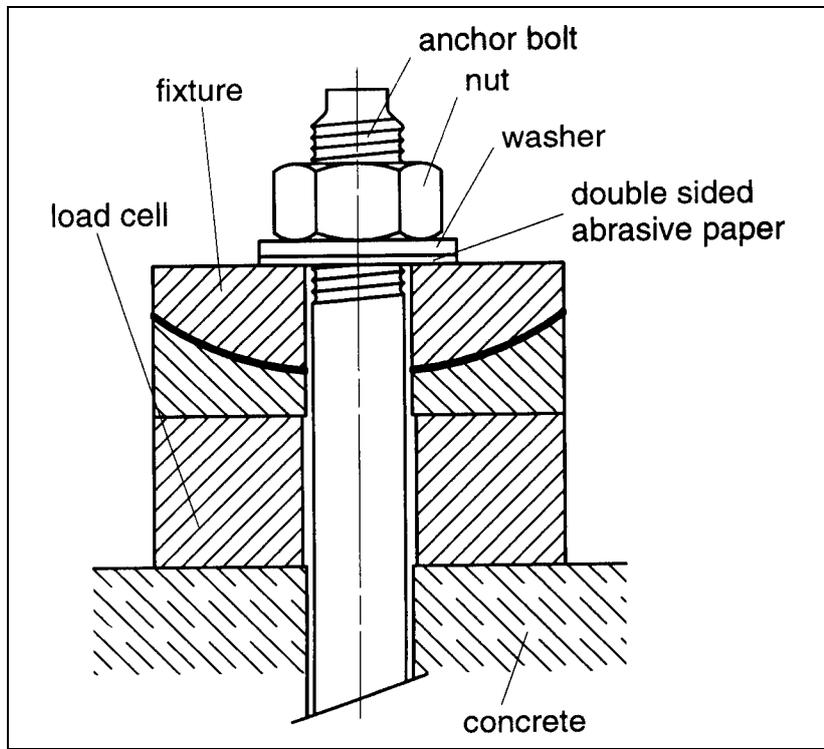
Figure D.8 Example for torque test (schematic)
