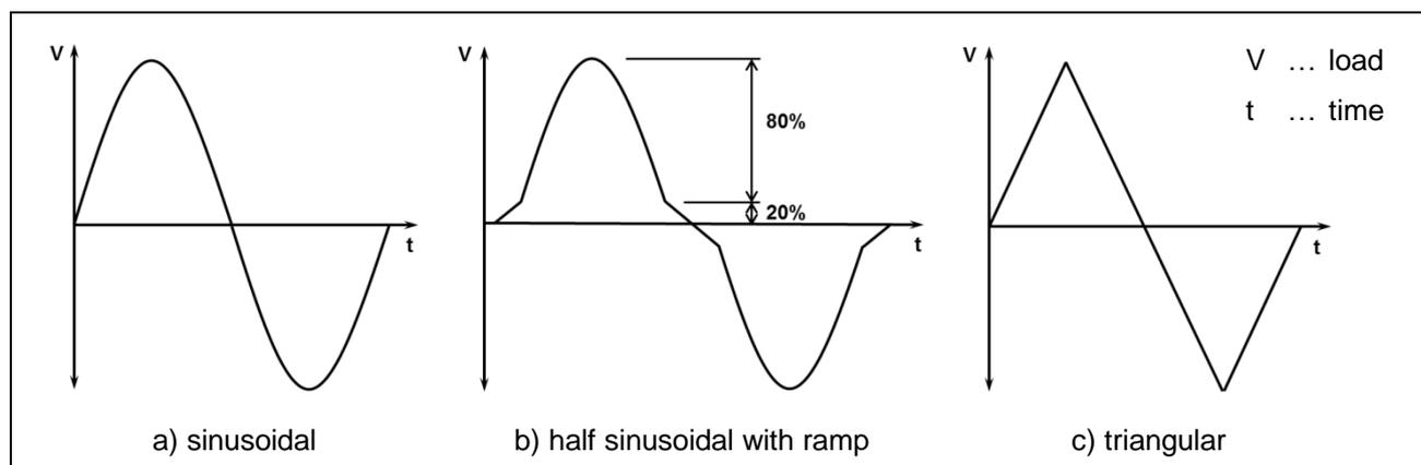
Figure E.12 Permitted seismic shear cycle C2.4
