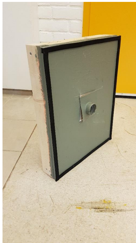
Figure F.1. Test piece of 2 layers of 13 mm gypsum fixed to a frame of steel or wood before and after application of membrane.
