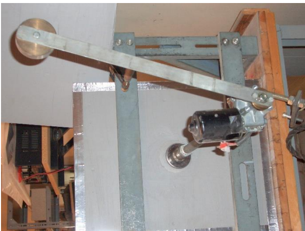
Figure F.5. Device for testing of bushings to dynamic load Note: the photo is of an earlier device giving a more harsh load.
