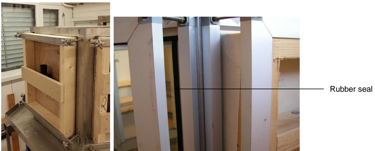
Figure F.2. Sealing with a soft (hollow) rubber profile.
