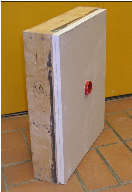
Figure F.1. Test piece of 2 layers of 13 mm gypsum fixed to a frame of steel or wood before and after application of membrane.
