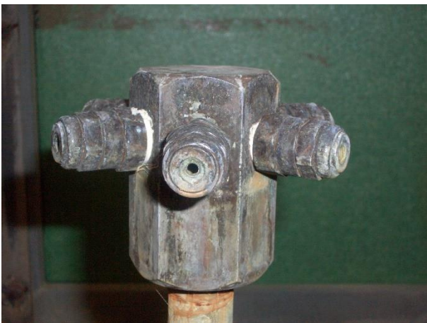
Figure F.4. Nozzles for water spraying – close up and overview.
