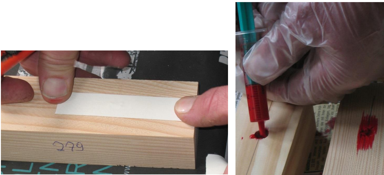
Fig. 3: Sealing a specimen and pouring the dye.
