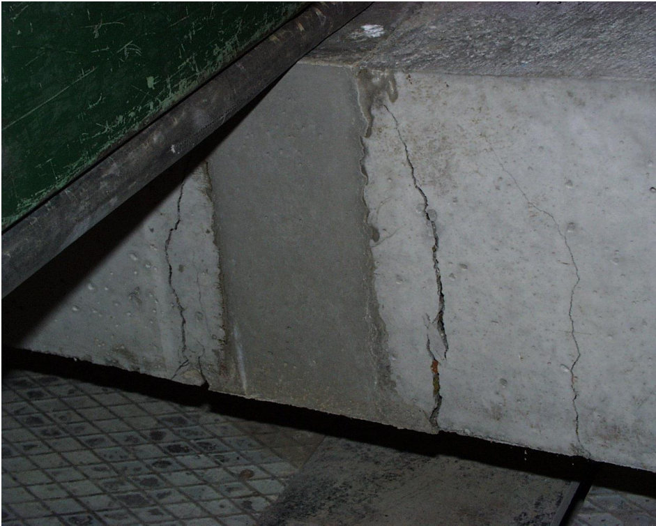
Figure 8: Beam specimen from fig. 7 in 3-point bending.
