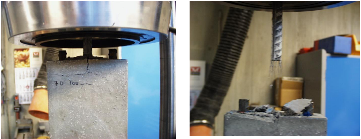
Figure 4: Pull-out of specimen with 100 mm embedment length of \varnothing 16 bar tested at 3 days.
