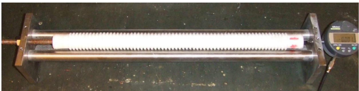
Figure 2: Experimental set-up for measurement of autogenous shrinkage using micrometer gauge.
