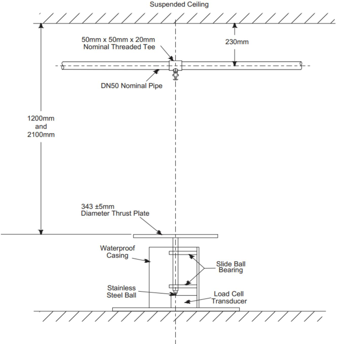
**Figure F.1: Thrust measurement test apparatus (side view)**
