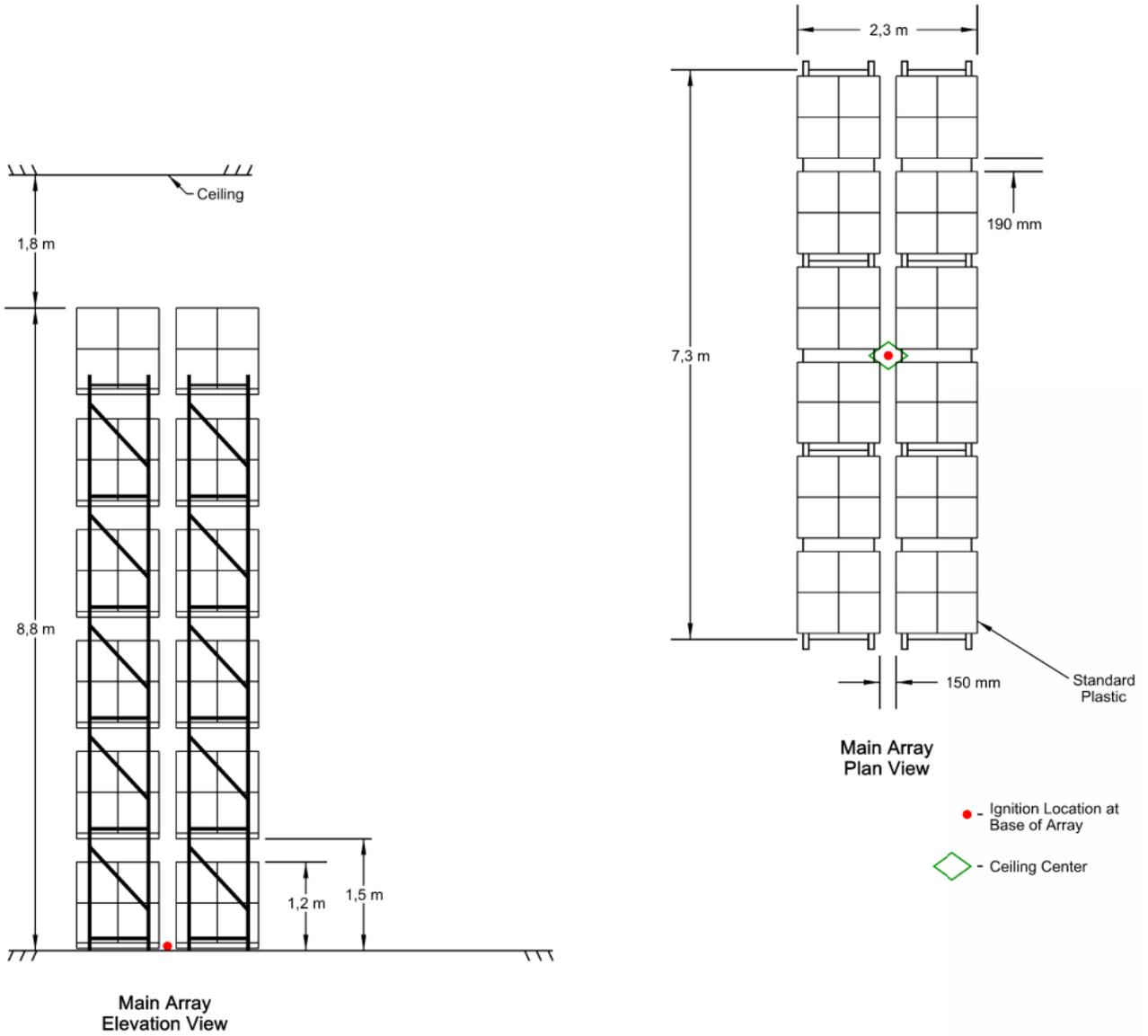
Figure A.1.5 Full scale fire test array for ESRF K202 upright, Test E
