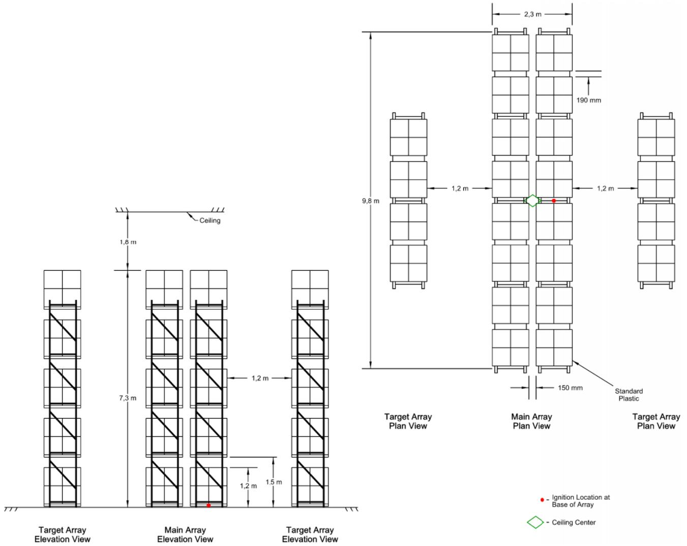
Figure A.6.1 Full scale fire test array for ESRF K202 and K240 pendent, Test A
