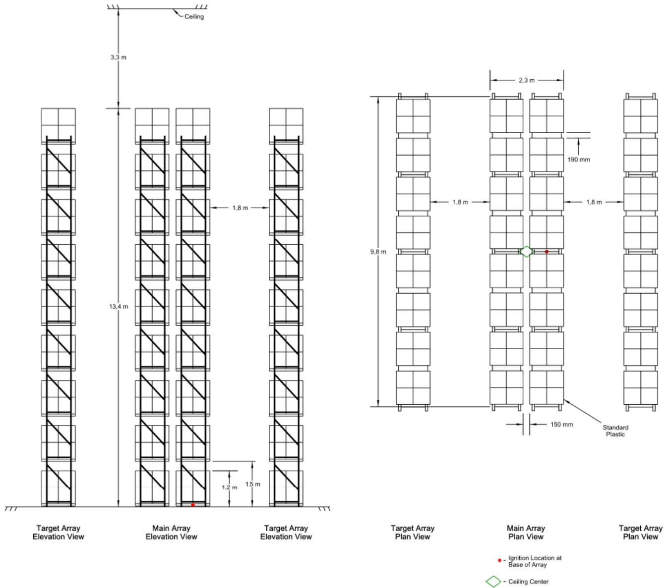
Figure A.5.2 Full scale fire test array for ESFR K480 pendent, Test B and C
