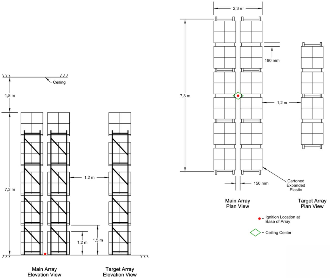
Figure A.1.2 Full scale fire test array for ESRF K202 upright, Test B
