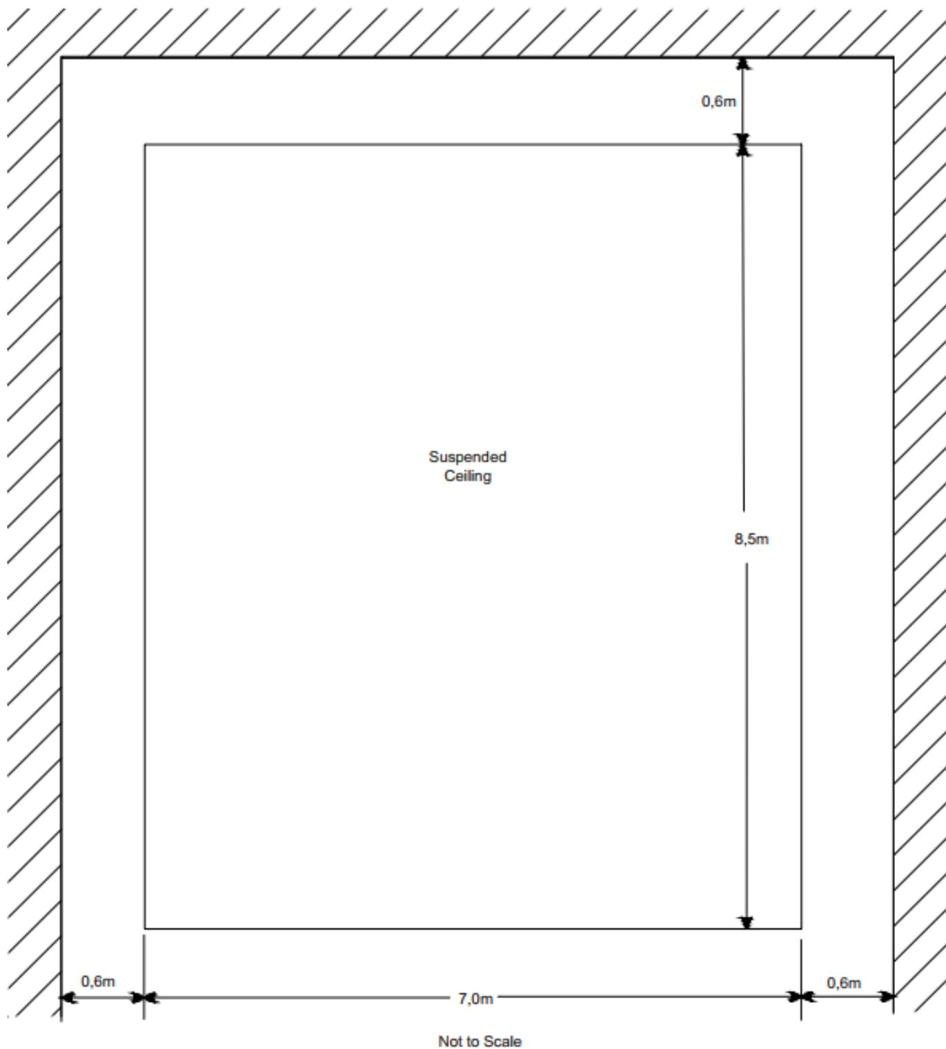
Figure B.1 Water distribution collection apparatus minimum enclosure dimensions (plan view)
