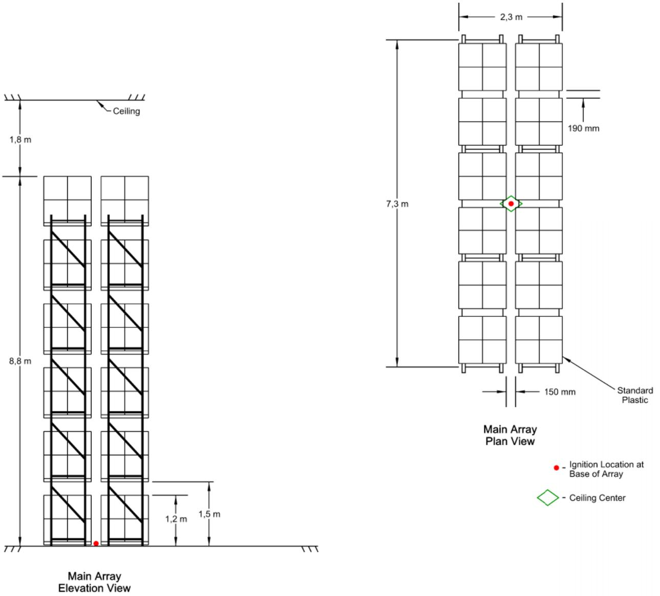
Figure A.2.5 Full scale fire test array for ESRF K240 upright, Test E
