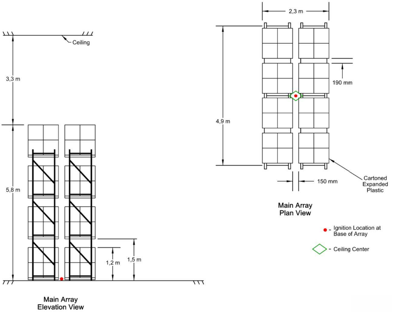
Figure A.1.1 Full scale fire test array for ESRF K202 upright, Test A
