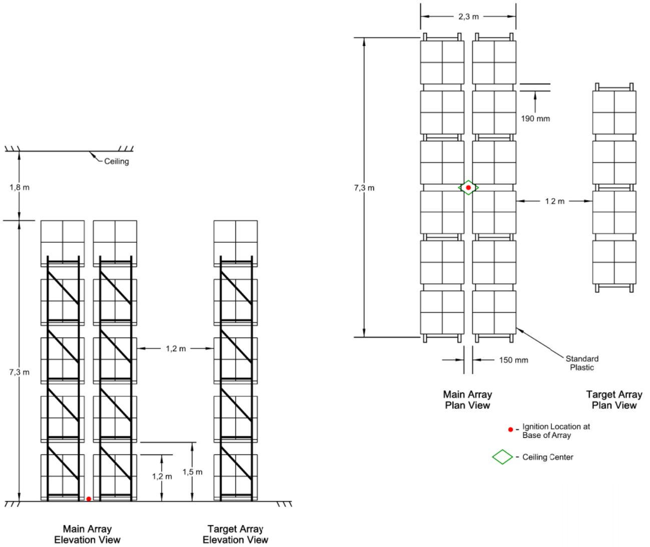
Figure A.1.3 Full scale fire test array for ESRF K202 upright, Test C
