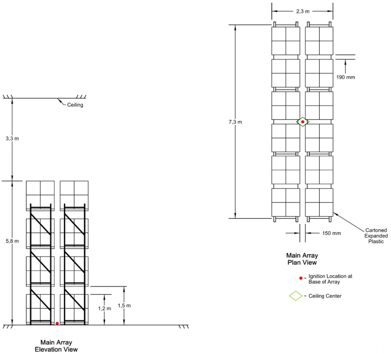
Figure A.2.1 Full scale fire test array for ESRF K240 upright, Test A
