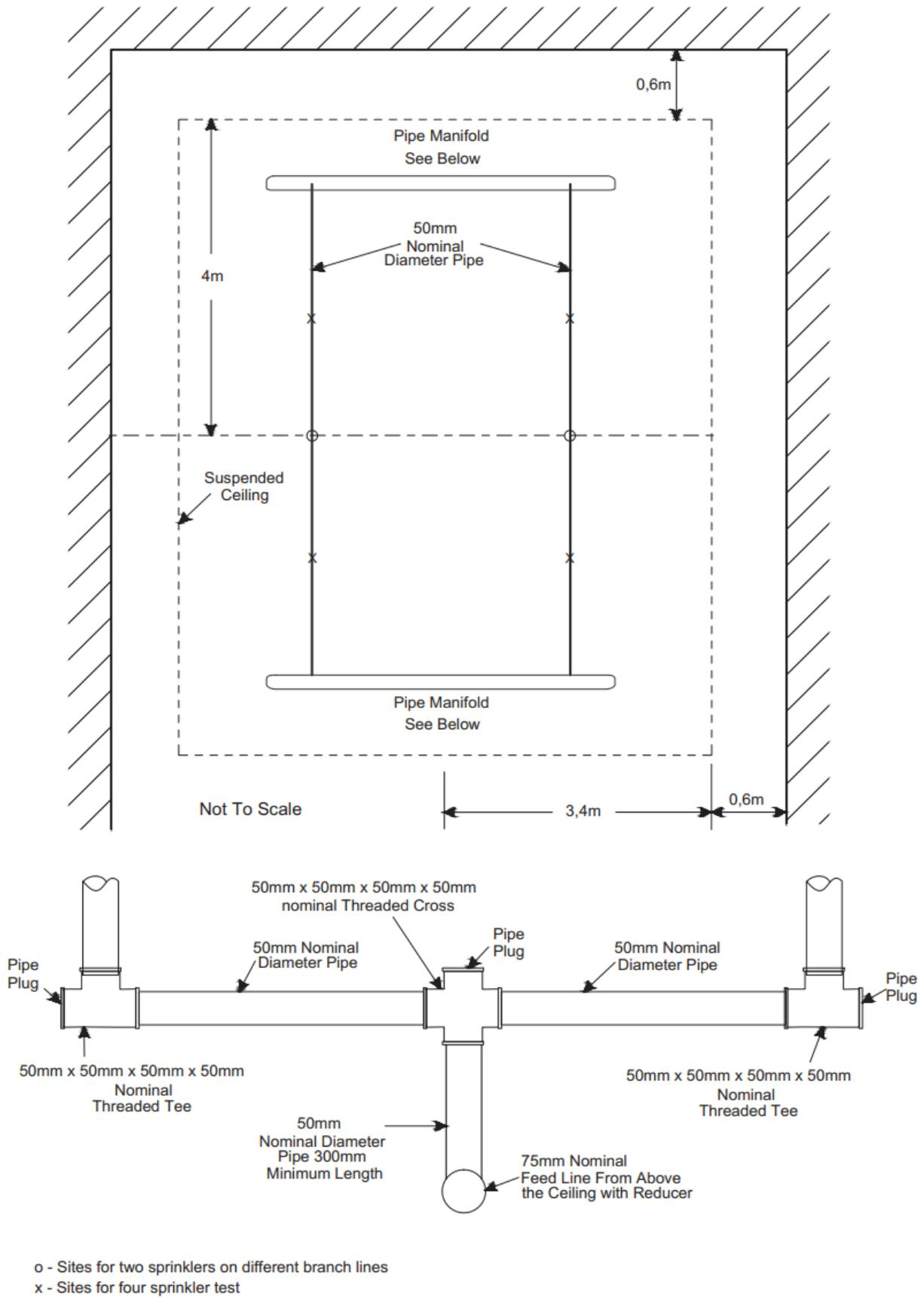
**Figure B.4** Water distribution collection apparatus multiple sprinkler piping configuration (plan views)
