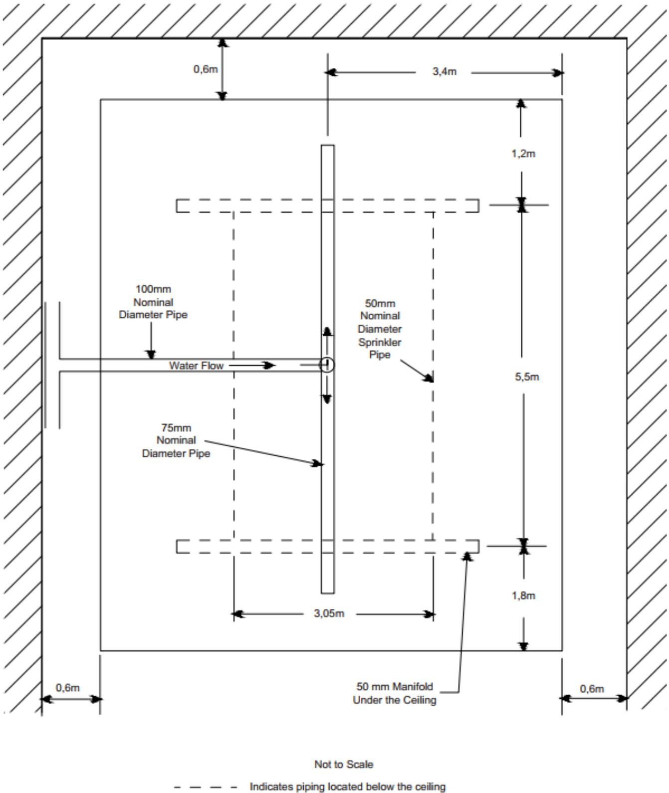
Figure B.2 Water distribution collection apparatus overhead piping configuration (plan view)
