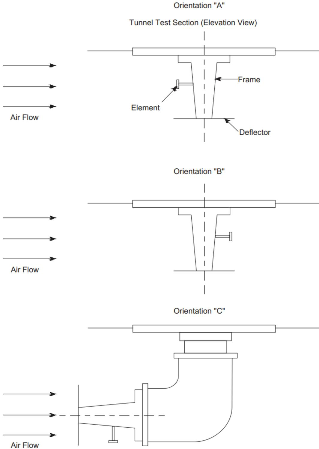
Note: In the case where the sprinkler has a symmetrical heat responsive element and frame, position "A" would be the same as position "B". Testing in both positions is not required.
