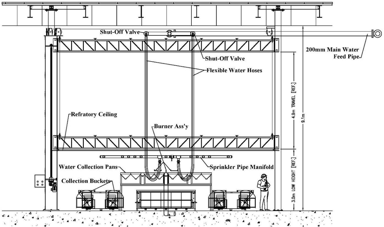
**ADD Apparatus Elevation View**
