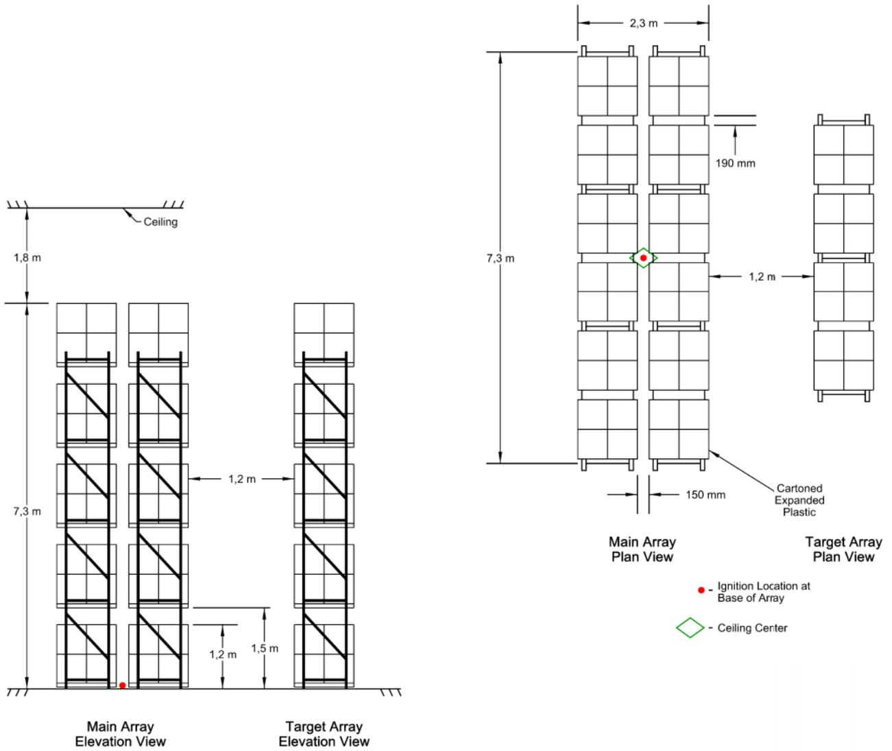
Figure A.2.2 Full scale fire test array for ESRF K240 upright, Test B
