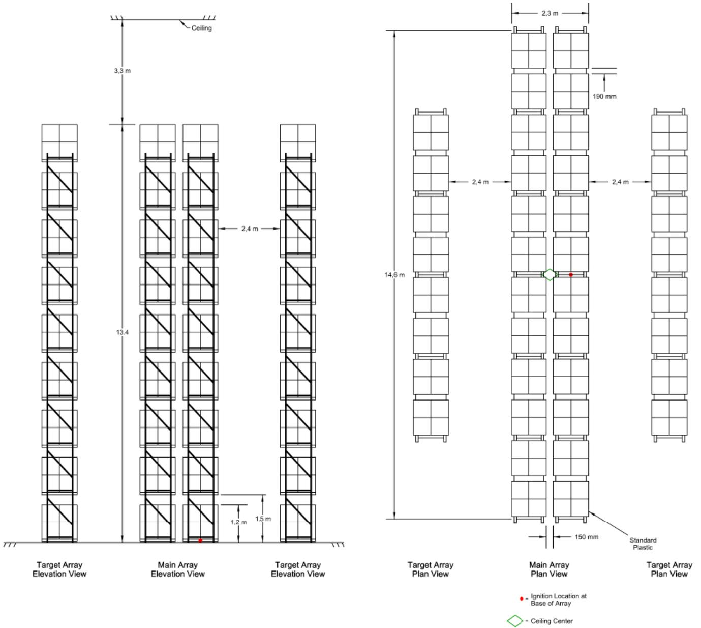
Figure A.4.2 Full scale fire test array for ESRF K400 pendent, Test B and C
