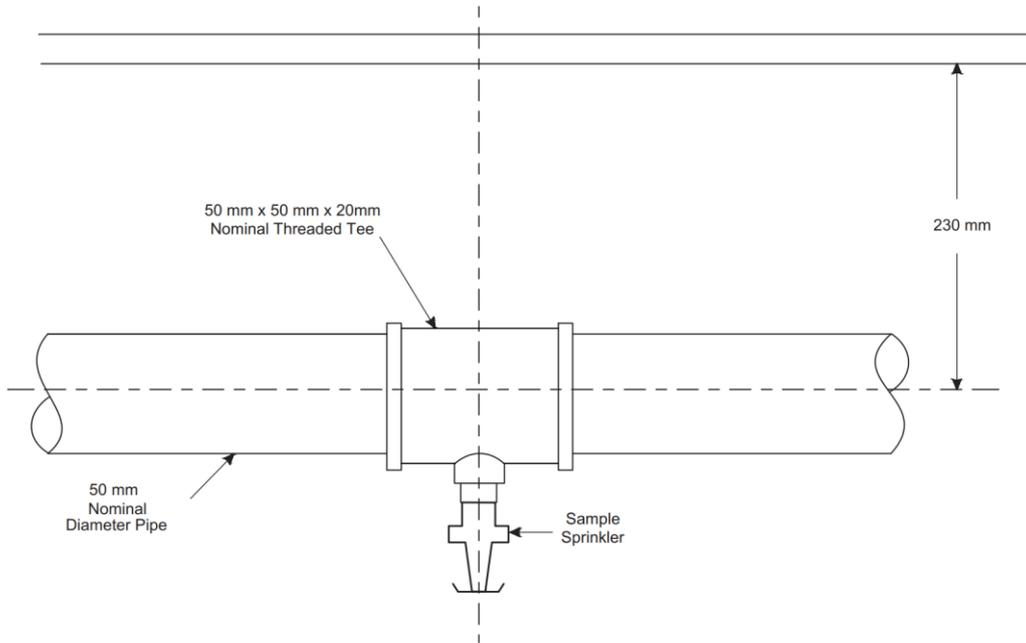
**Figure B.5 Water distribution collection apparatus piping detail**
