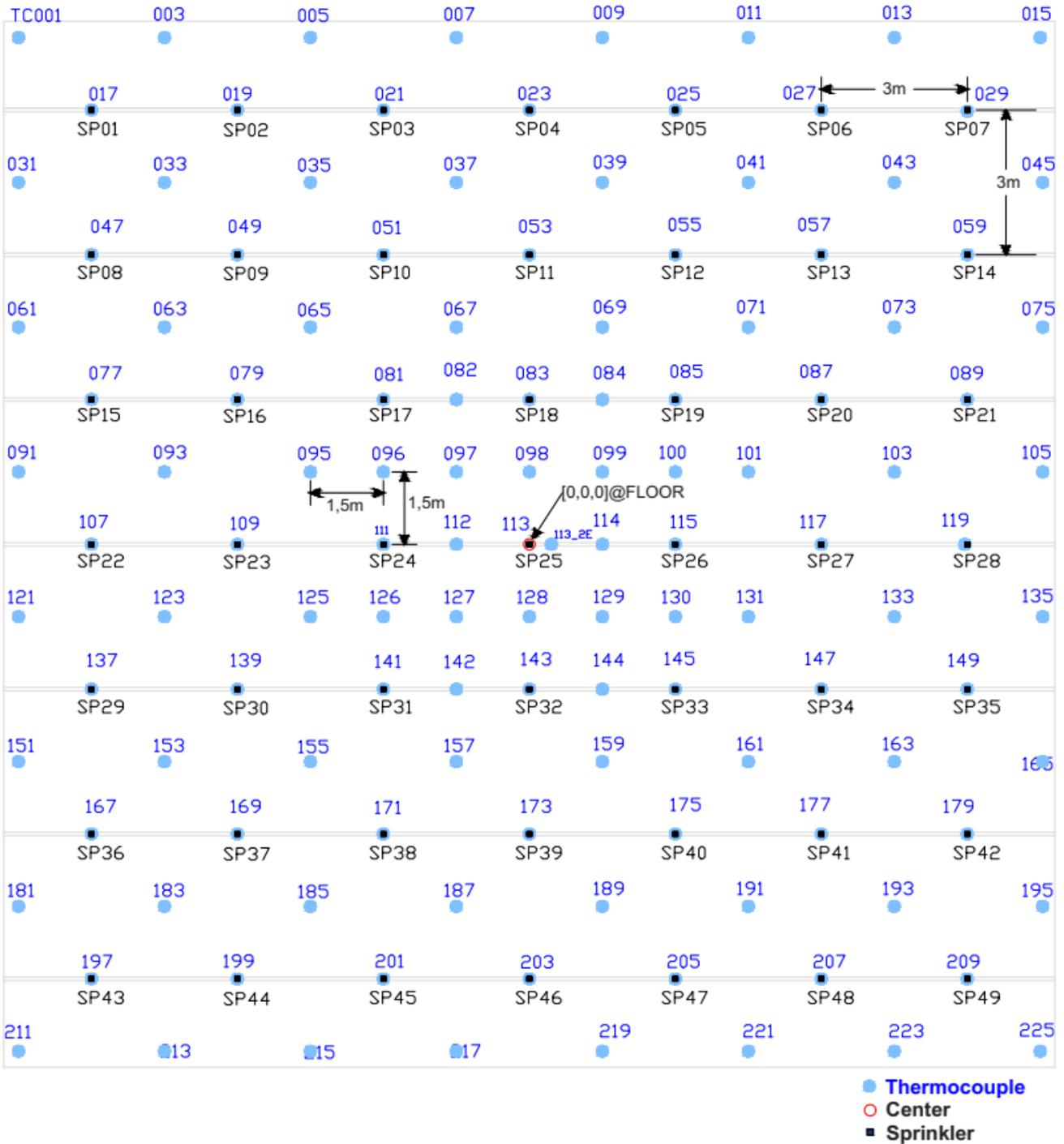
Figure A.1.6 Typical thermocouple layout
