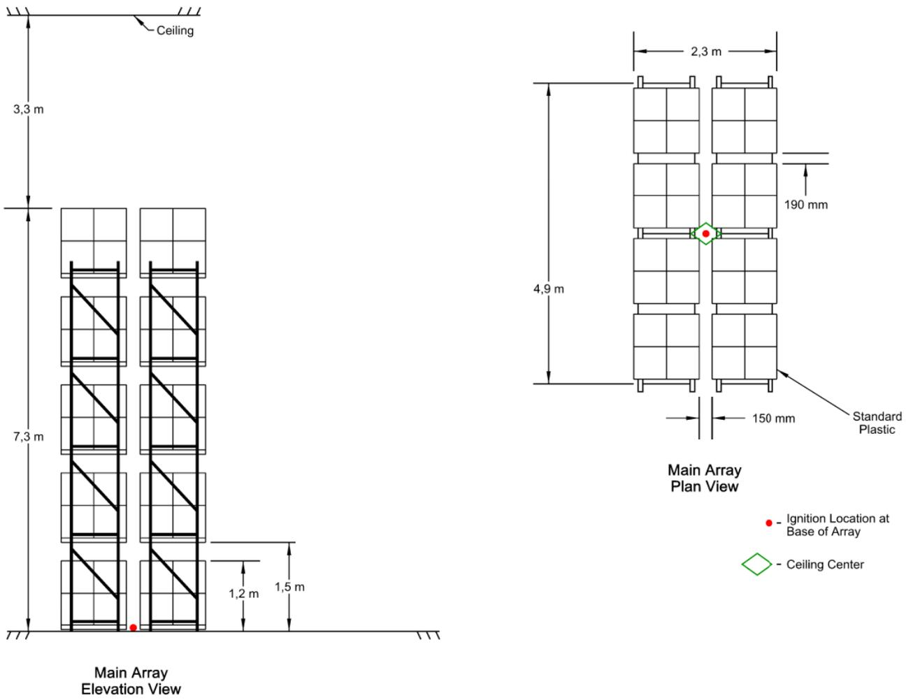
Figure A.2.4 Full scale fire test array for ESRF K240 upright, Test D
