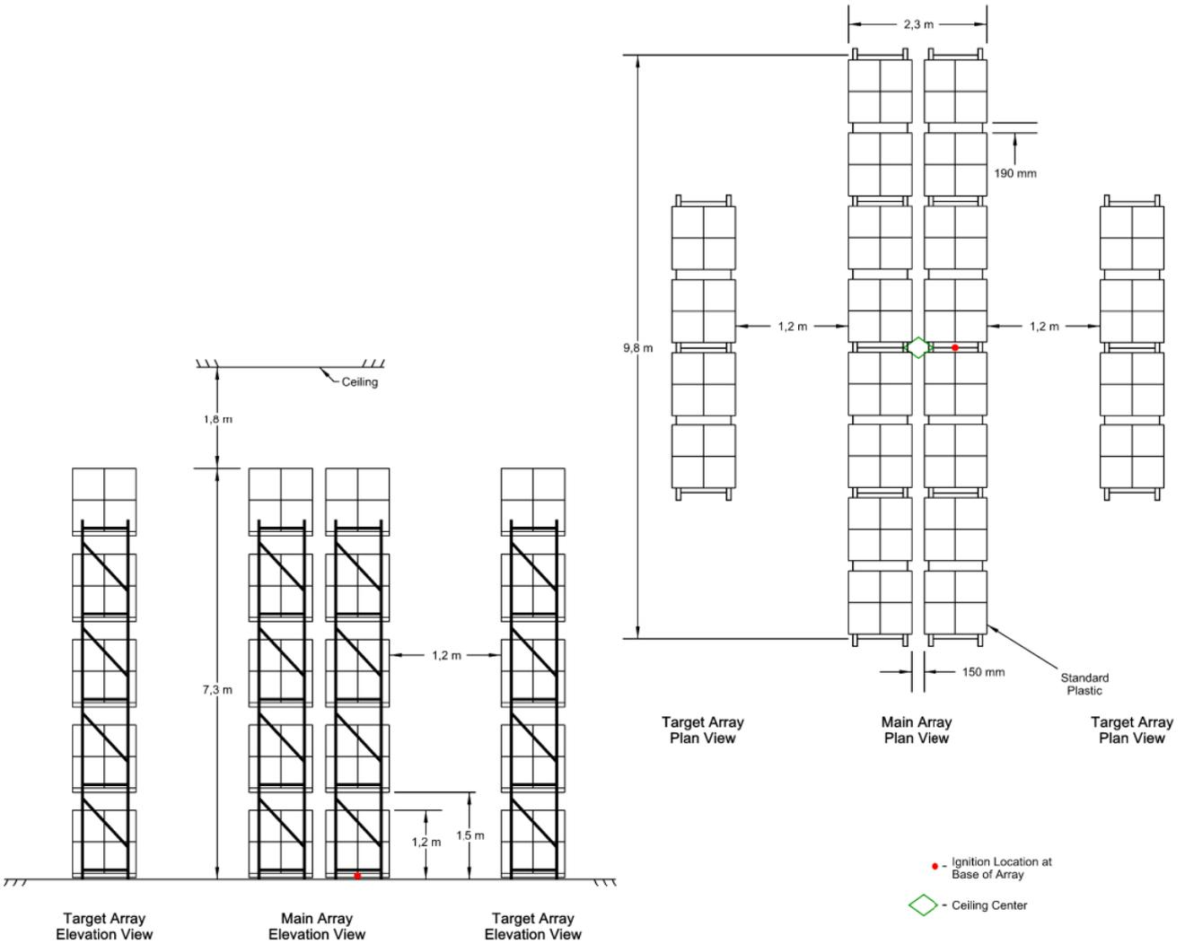
Figure A.3.1 Full scale fire test array for ESRF K325 and K360 pendent, Test A
