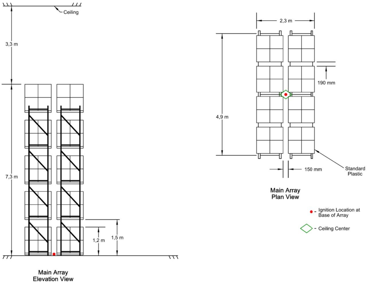
Figure A.1.4 Full scale fire test array for ESRF K202 upright, Test D
