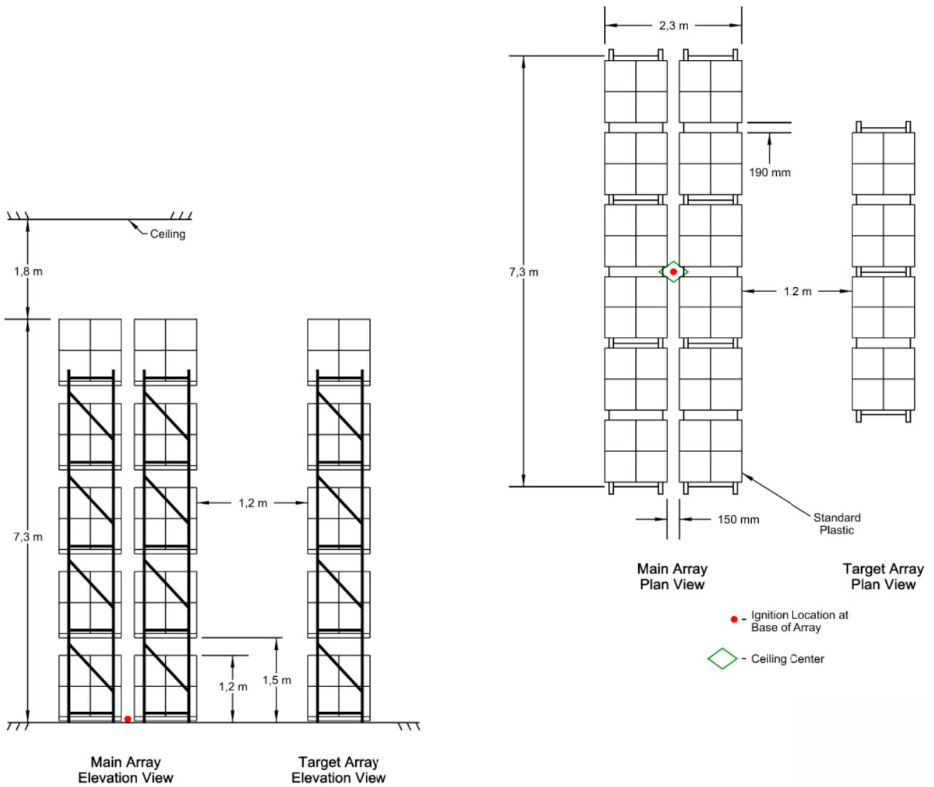
Figure A.2.3 Full scale fire test array for ESRF K240 upright, Test C
