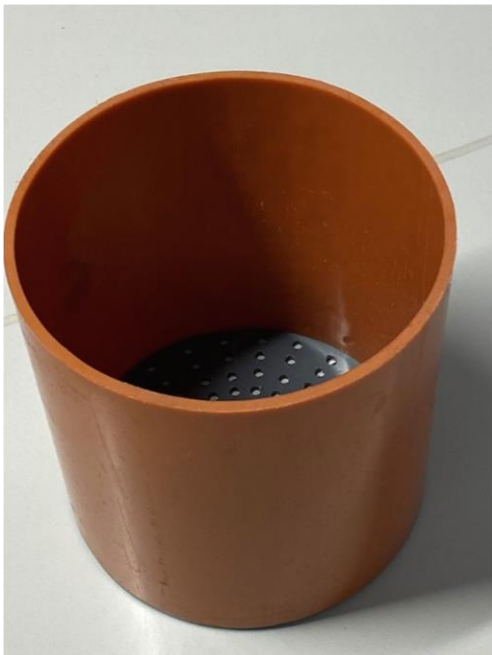
Figure G.2.1: Example of a cylindrical plastic container (with a perforated base) Source: Daniel Westerholt
