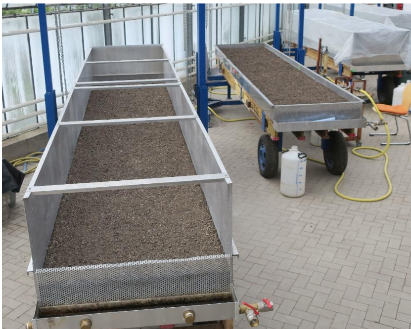
Figure D.2.1: Example of measuring tables (which can be made of other material, e.g., wood with sealing) Source: Daniel Westerholt
