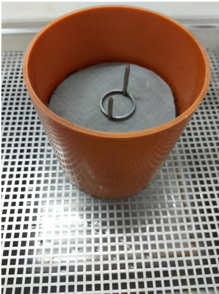
Figure F.3.1: Cylindrical plastic container with geotextile filter fleece, sieve mesh and measuring probe ring (on the top of the specimen) Source: Daniel Westerholt
