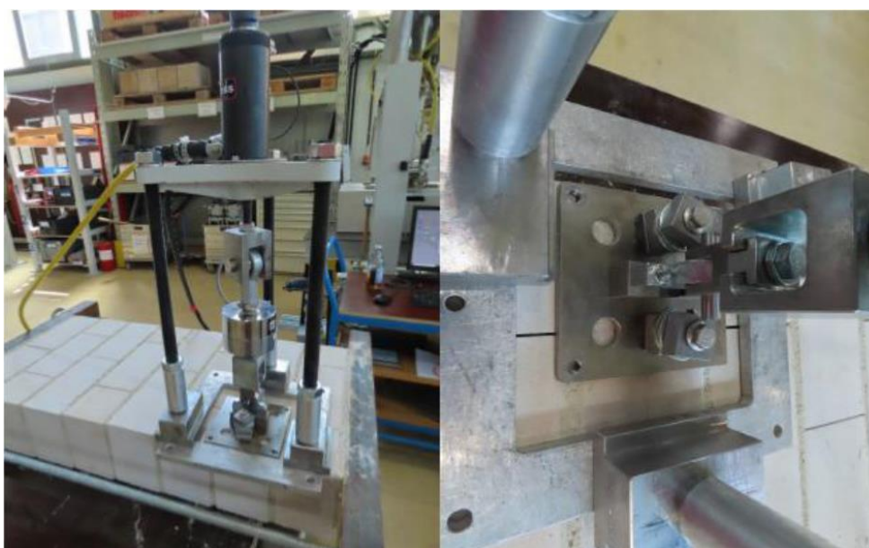
Figure A.5.2.7: Example of test setup for tension tests of a double screw anchor group (test series A5sII)
