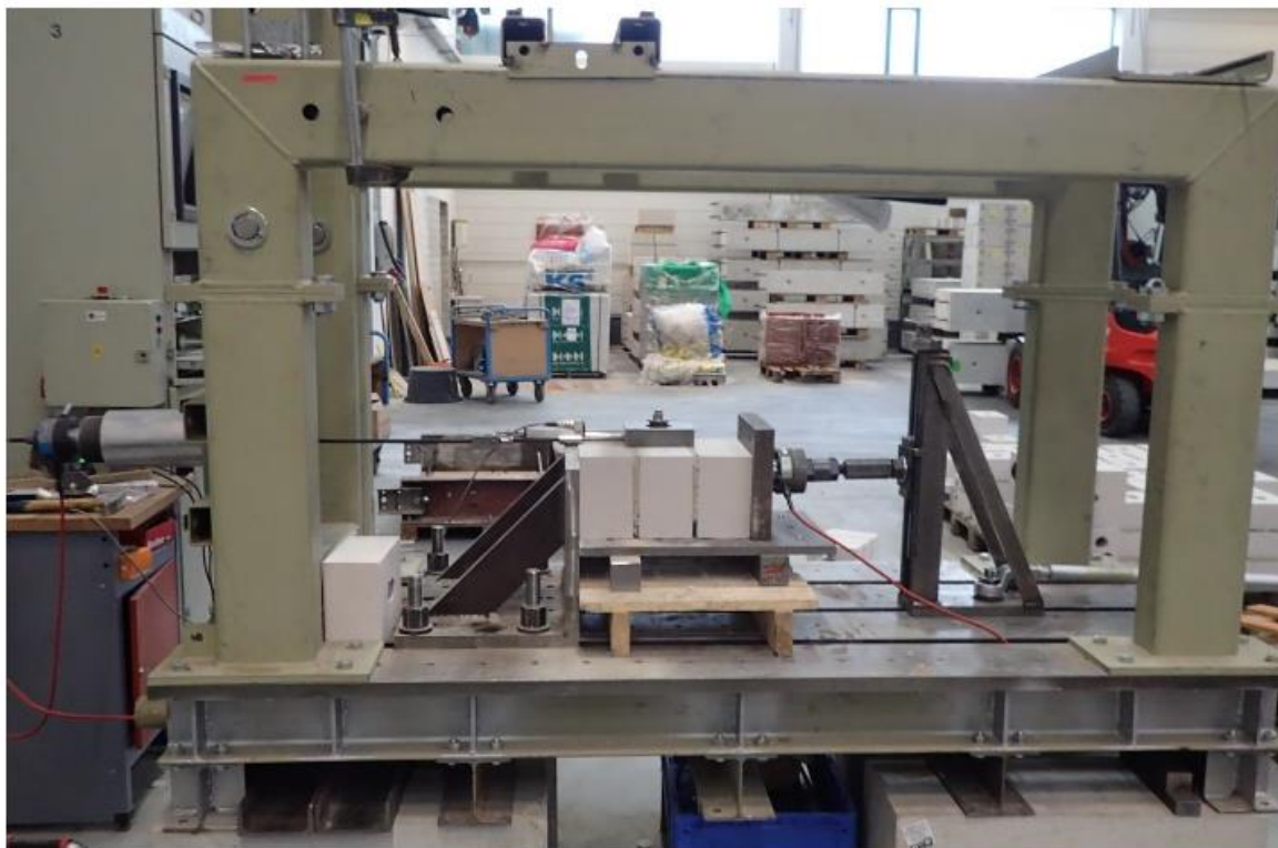
Figure A.5.3.2: Example of test setup for shear tests with shear loading parallel to the edge (test series A4II)
