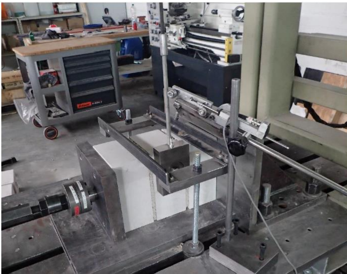
Figure A.5.3.3: Example of the test setup for shear tests with shear loading perpendicular to the edge (test series A4 \perp )
