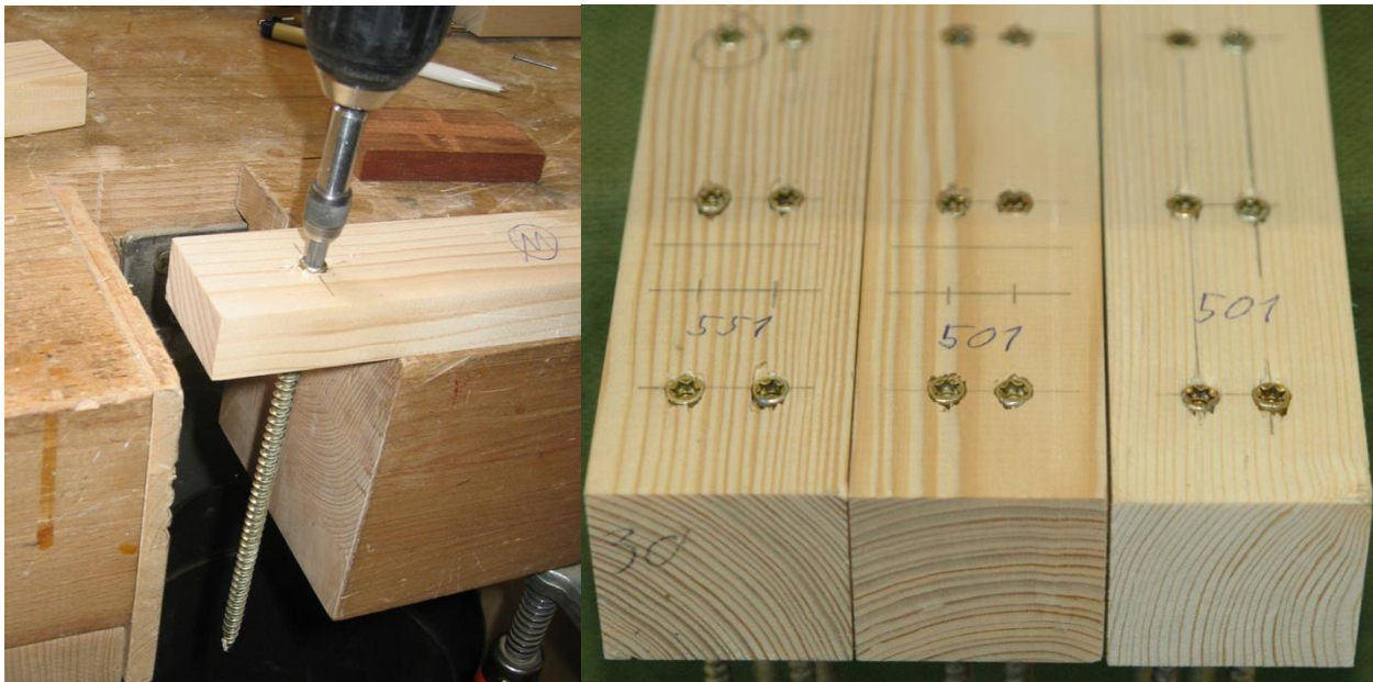
Fig. 2: Inserting a screw (left), specimens with 2 rows of 3 screws (right).
