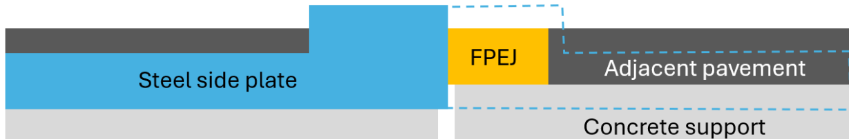
Figure B.4.1: Side view of the test specimen – showing steel side plates used for its construction
