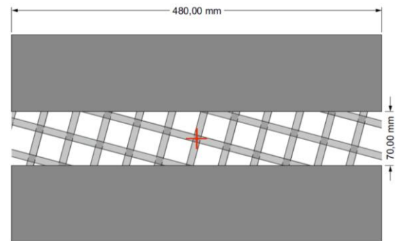
b) Clamping of the specimen with 15° rotation 11 md tensile bars are clamped
