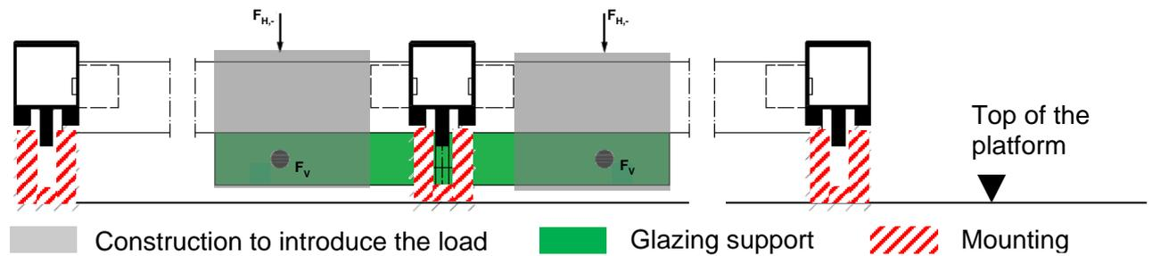
Figure B.7 Test setup and applied load direction (cruciform glazing support, double-sided combined load)
