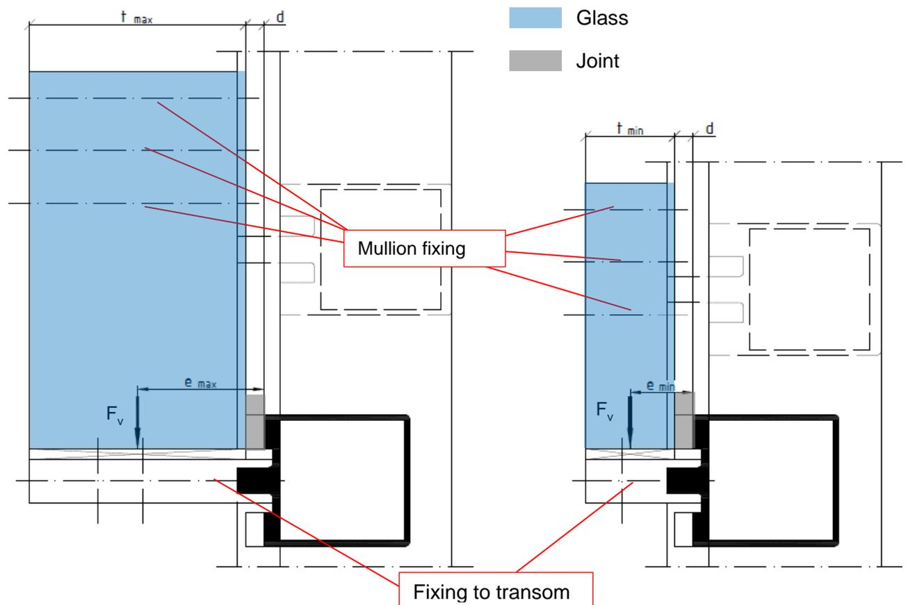
Figure B.1 Eccentricities for minimum and maximum glass thickness (cruciform glazing support)
