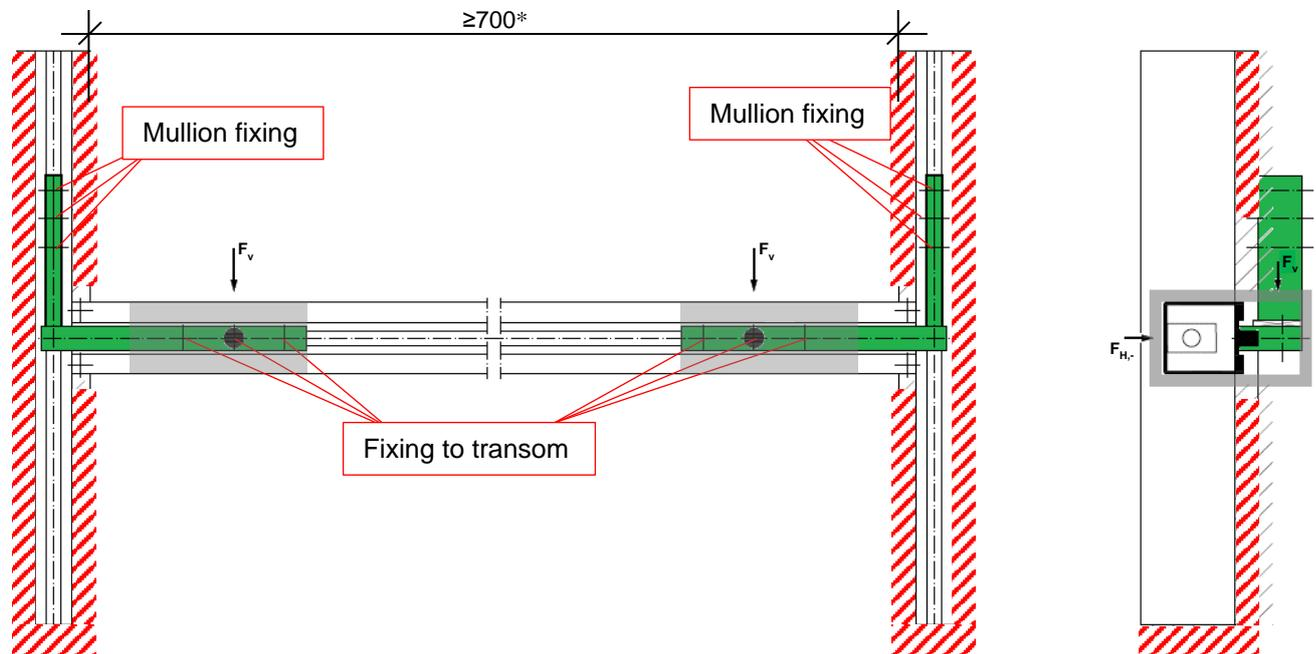
**Front view test set-up:**
