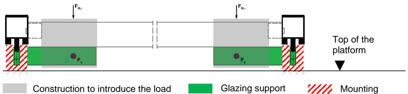
Figure B.8 Test setup and applied load directions (cruciform glazing support, one-sided combined loads)
