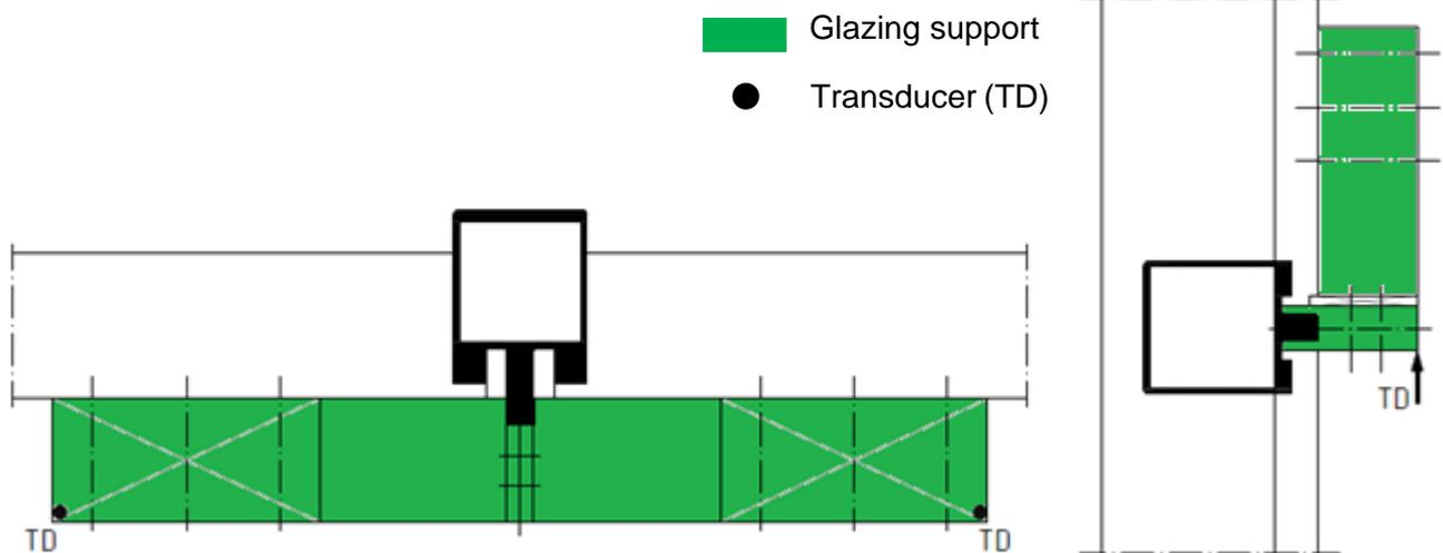
Figure B.2 Position of the transducers
