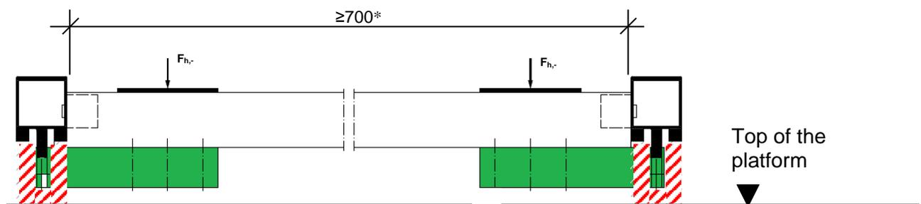
\*dimensions according to the H test samples in EN 16758
