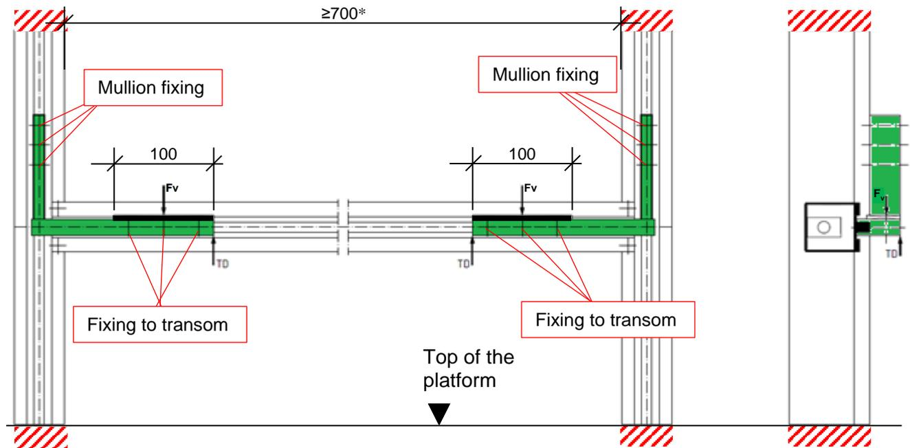
\*dimensions according to the H test samples in EN 16758
