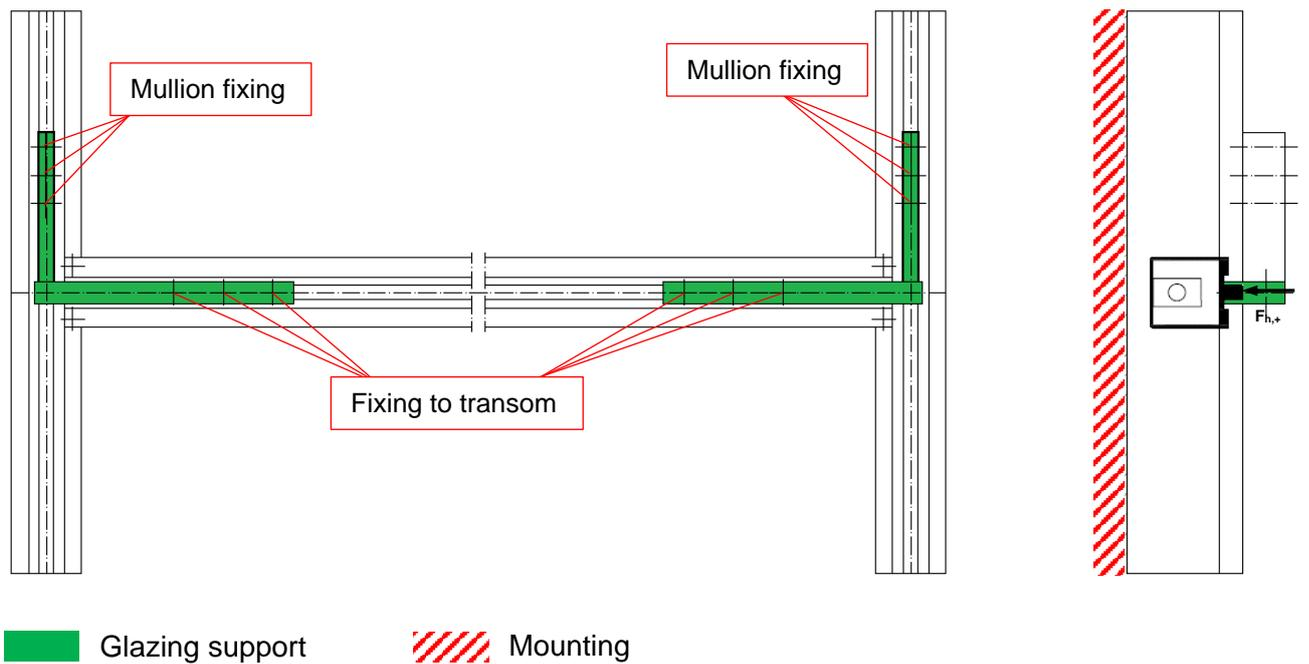
Figure B.6 Test setup and position of the load (wind pressure)
