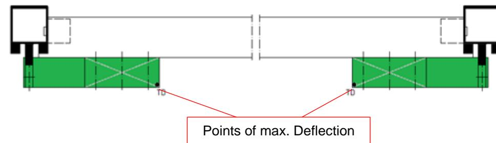
■ Glazing support    ▨ Mounting    ● Transducer (TD)
