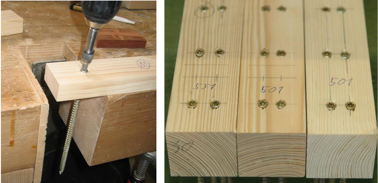
Fig. 2: Inserting an insert (left), specimens with 2 rows of 3 inserts (right).
