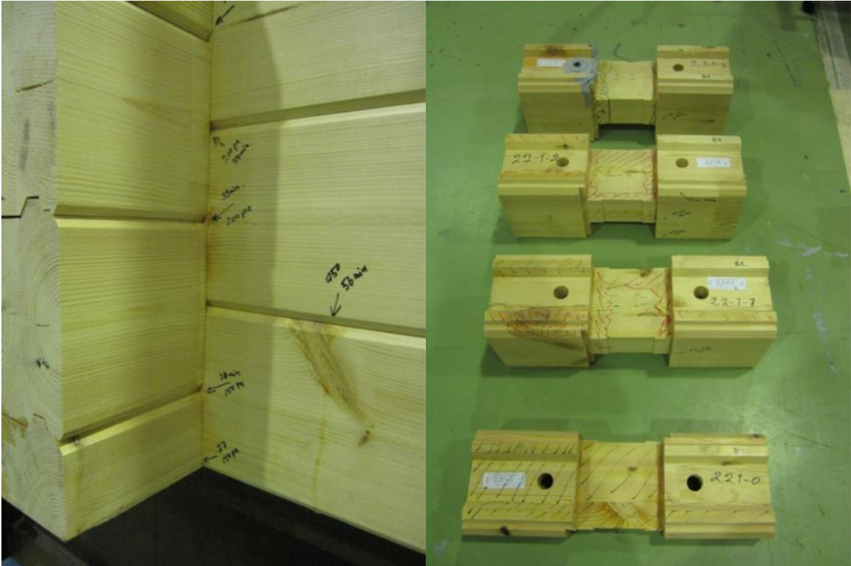
Figure B.4: Left: Marking of water leakage points and the time and pressure when the leakage has started in watertightness test. Right: Example of marking the wet areas to logs after dismounting of the specimen in watertightness test.
