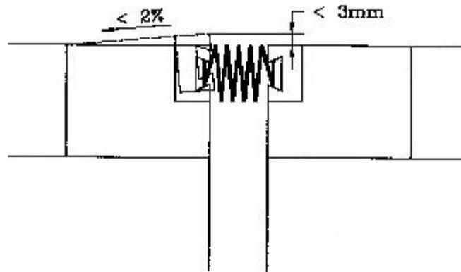
Figure 4: Level differences in the area of transition strip (if part of the kit)
