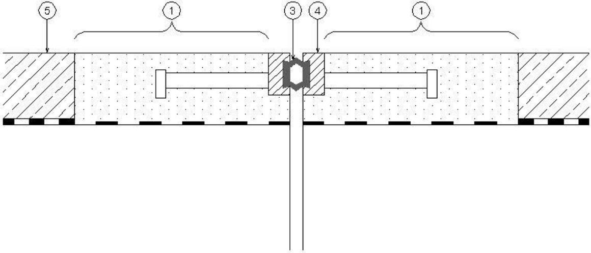
d) A combination of adhesion to the bridge deck concrete completed by fastening of reinforcement into holes
