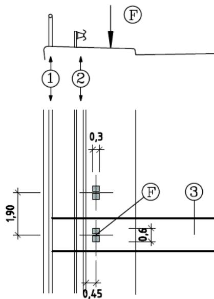
Key: ① Pedestrian parapet ② Safety barrier ③ Expansion joint  $F = A_d/2 = 100 \text{ kN}$
