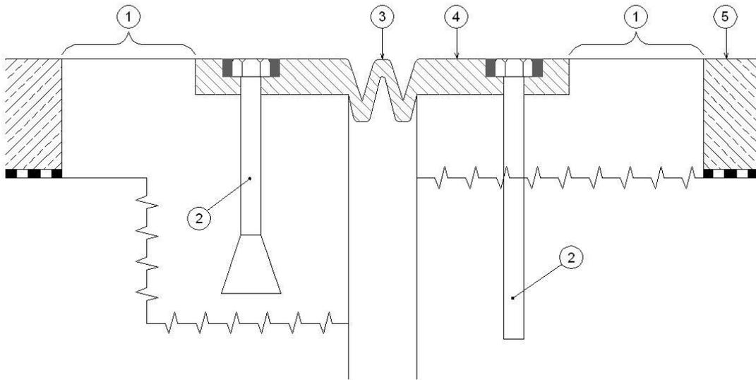
Type 2 the sealing element is held in place by clamping and/or adhesive or compression. The clamp to maintain the sealing element is generally in metal but it is possible to have this clamp in resin mortar or other material.
