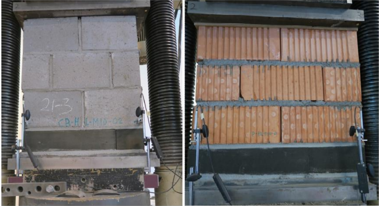
Figure 2.2.1.1: Examples of specimen for the compressive strength test, including details for deformation measurements
