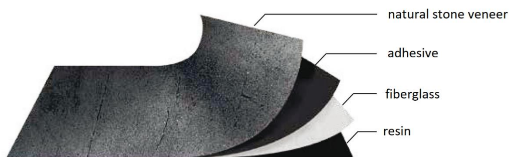
Figure 1.1.1 Typical layers of ultra-thin natural stone veneer sheets
