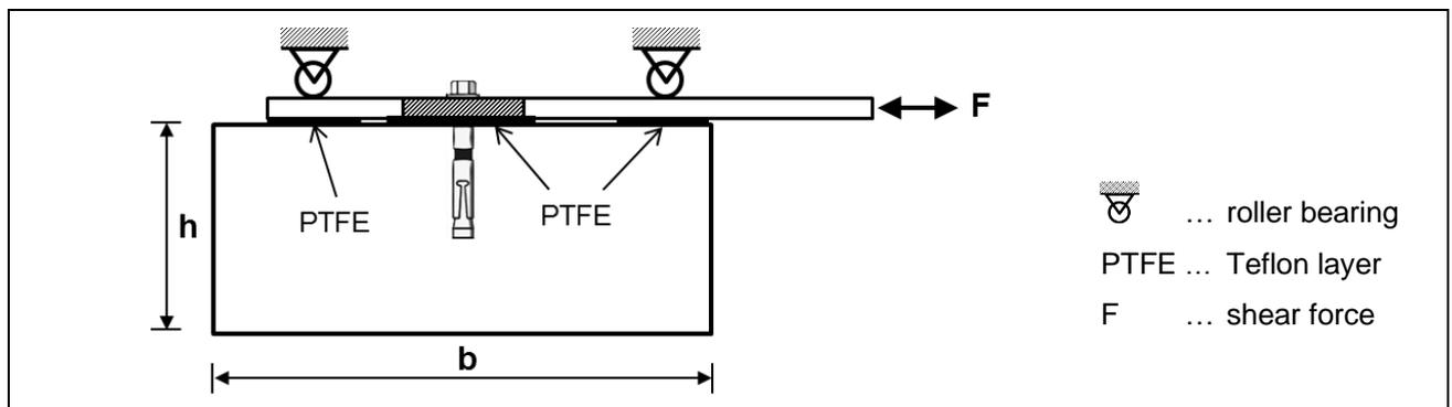
Figure E.5 Sketch of example for shear test setup with no significant friction forces
