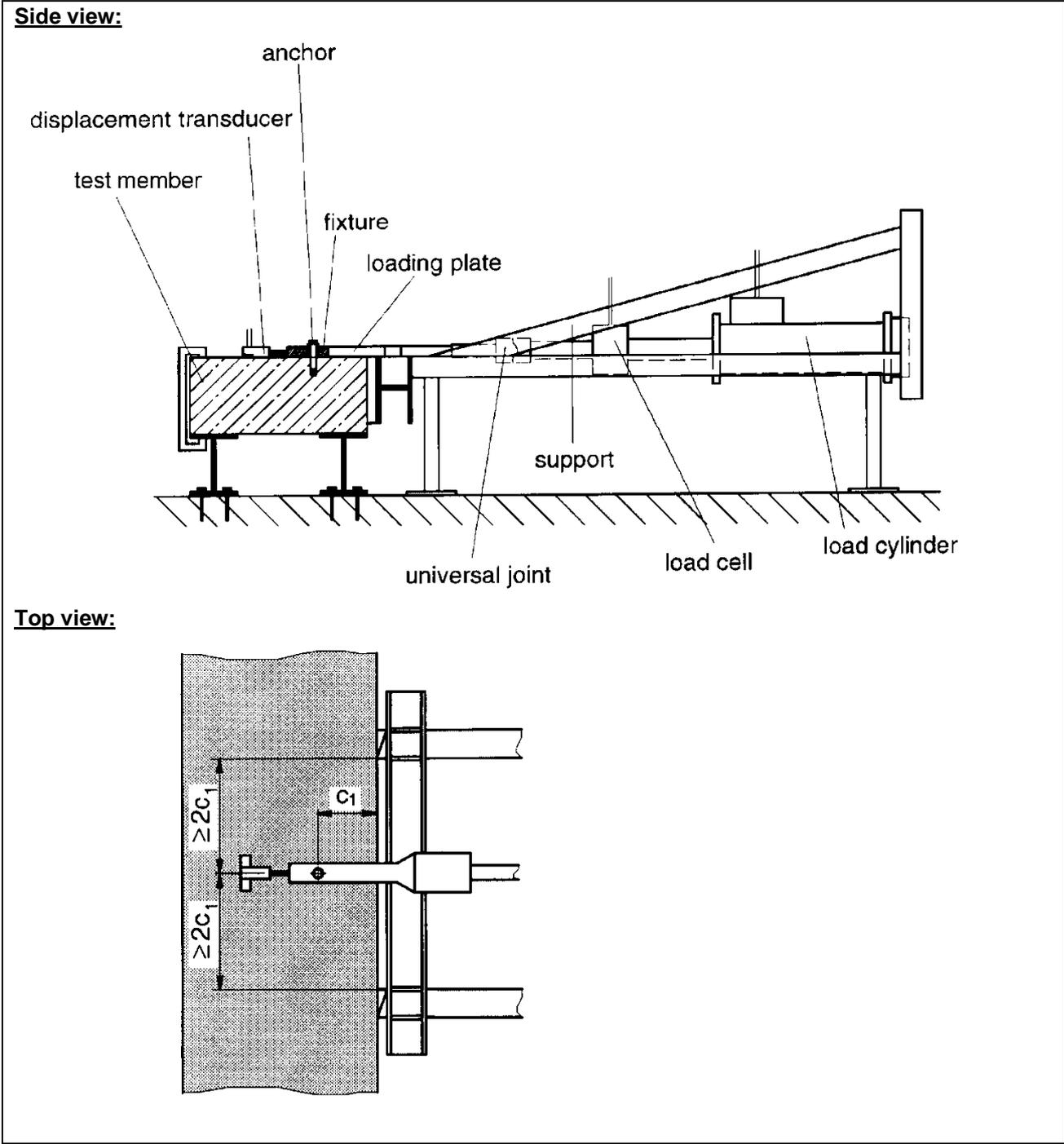
Figure D.7 Example of a shear test rig
