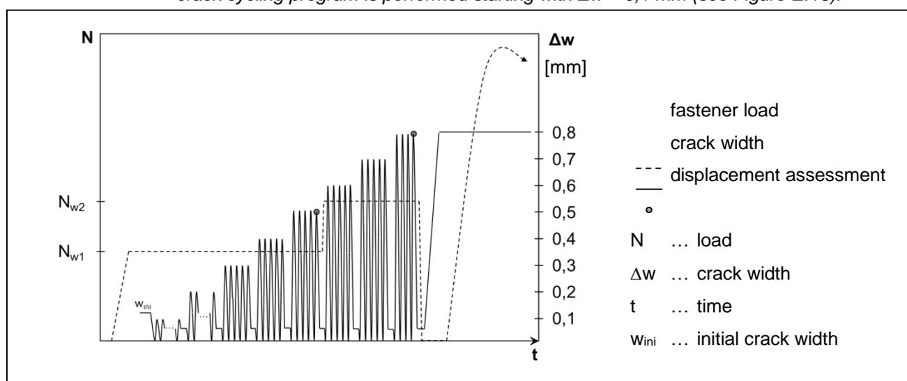
Figure E.13 Schematic test procedure C2.5
