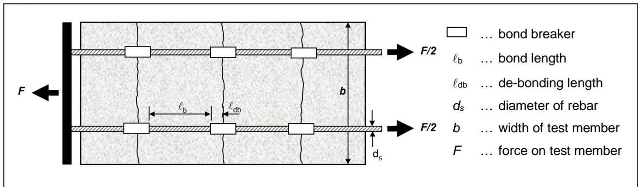
Figure E.2 Example for test member with bond breaking pipes on rebar (plan view)
