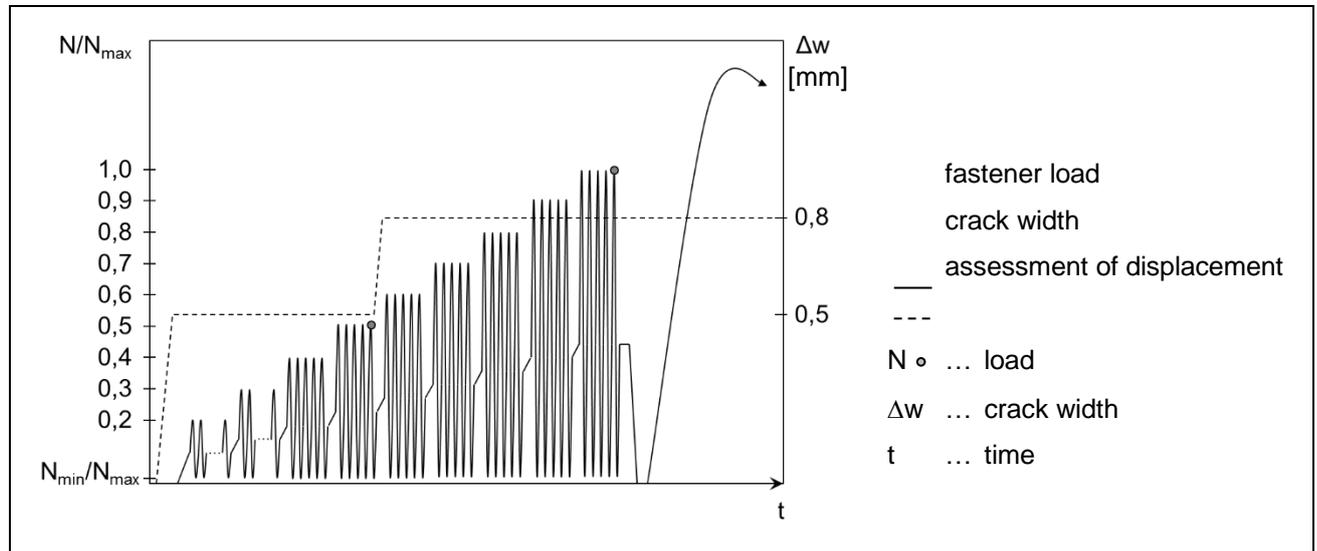
Figure E.10 Schematic test procedure C2.3
