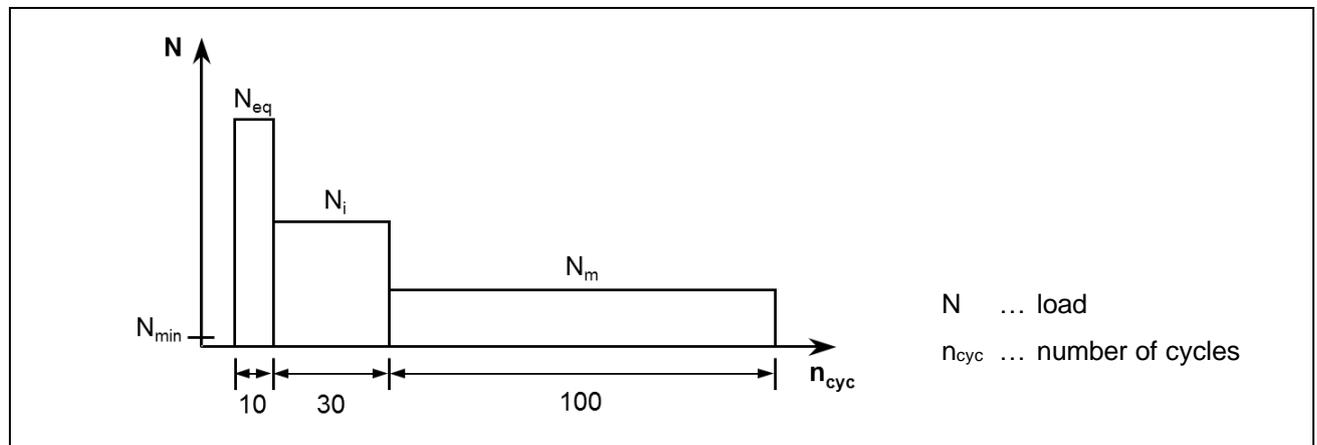
Figure E.7 Required loading history for test series C1.1
