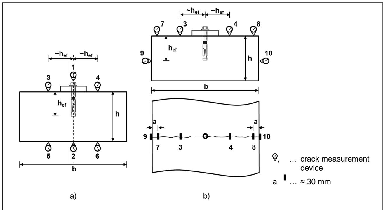
Figure E.3 Measurements to show fulfilment of the constant crack width requirement
