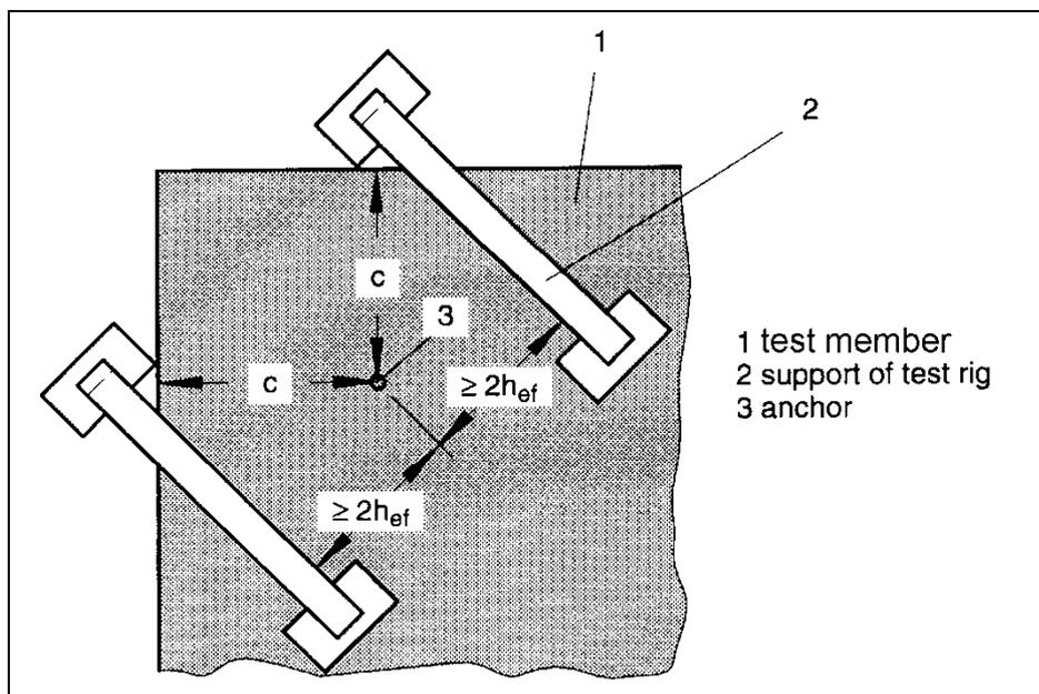
Figure D.9 Example of the test rig for tension tests on fasteners at a corner
