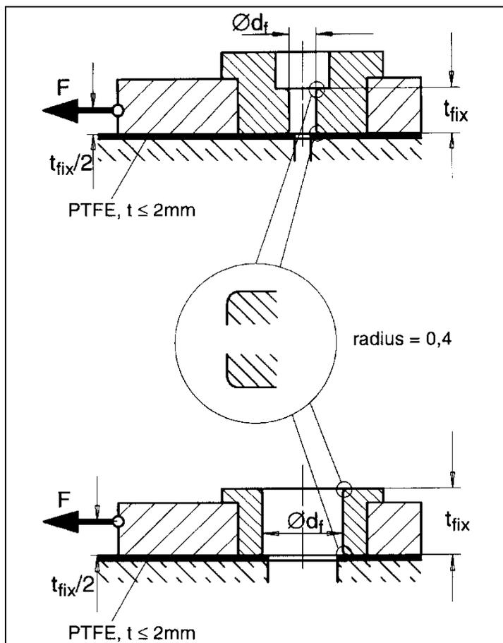
Figure D.6 Examples of shear test sleeves
