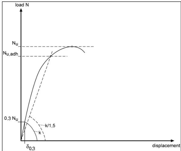
Figure A.3 Evaluation of load at loss of adhesion
