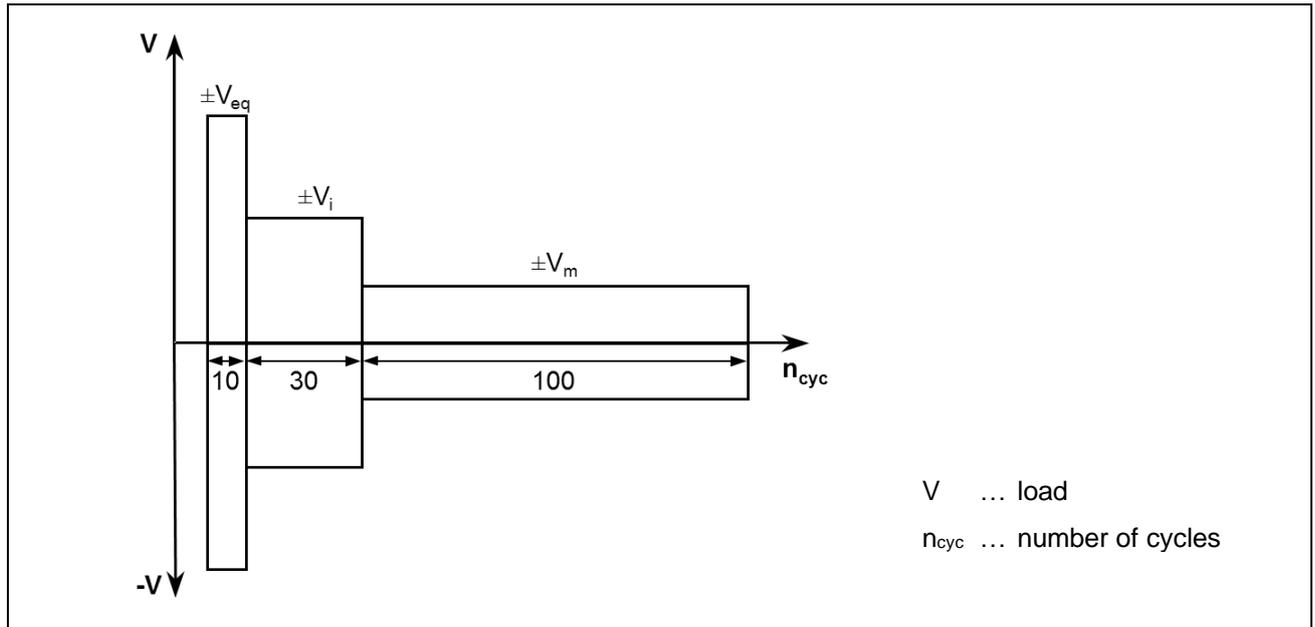
Figure E.8 Required load history for test series C1.2
