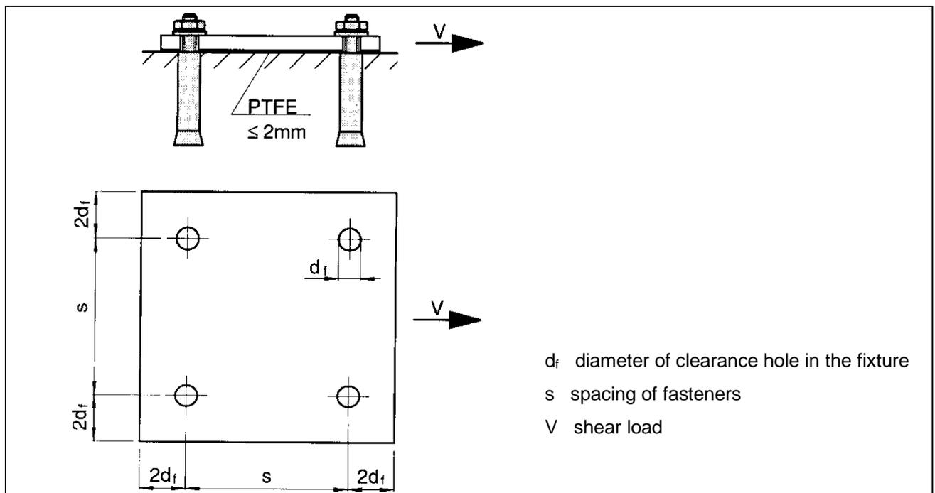
Figure D.13 Dimensions of fixture
