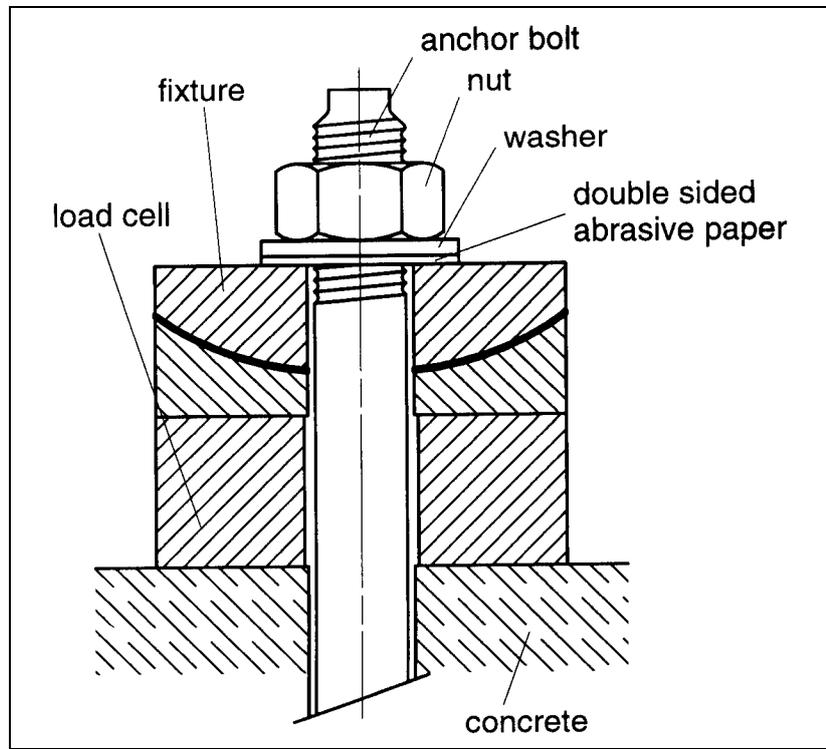
Figure D.8 Example for torque test (schematic)
