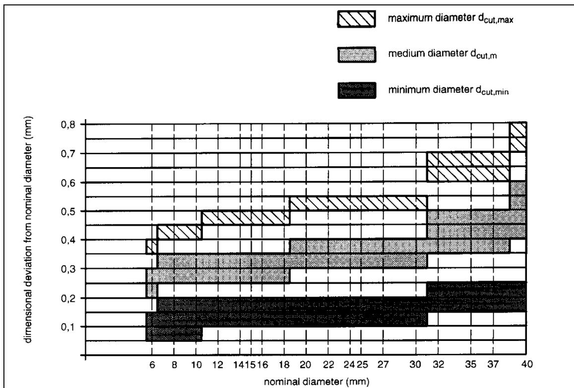
Figure D.5 Cutting diameter of hard metal hammer-drill bits
