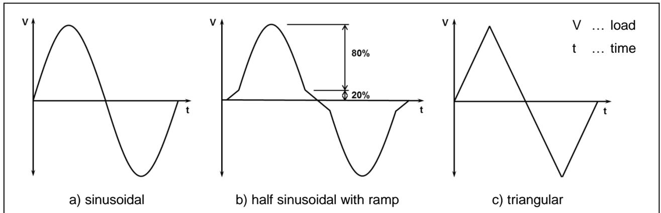
Figure E.12 Permitted seismic shear cycle C2.4
