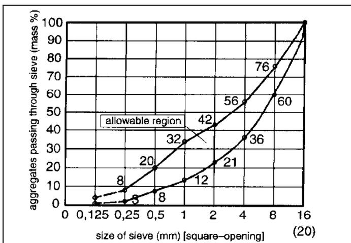
Figure D.1 Admissible region for the grading curve
