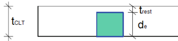
Figure 4: Embedment depth of the connector d_e in the cross laminated timber and remaining cross section t_{rest}
