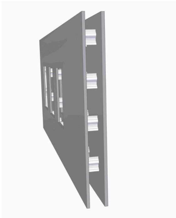
Figure 1: Precast concrete composite wall with point connectors
