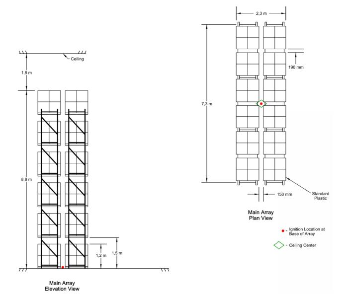
Figure A.1.5 Full scale fire test array for ESFR K202 upright, Test E
