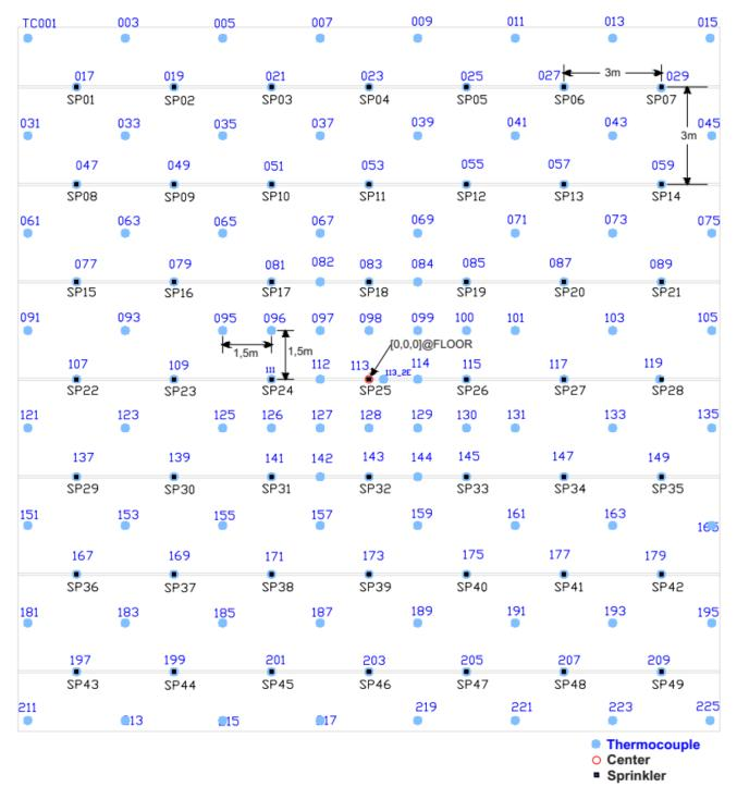
Figure A.1.6 Typical thermocouple layout
