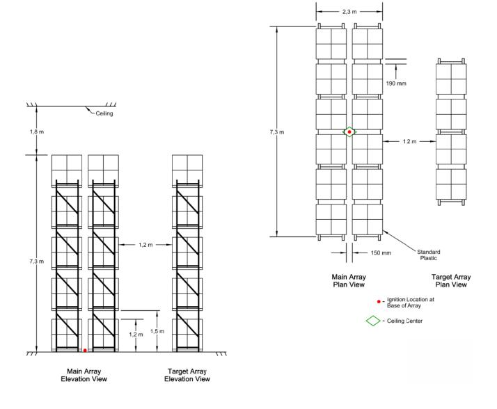
Figure A.2.3 Full scale fire test array for ESFR K240 upright, Test C
