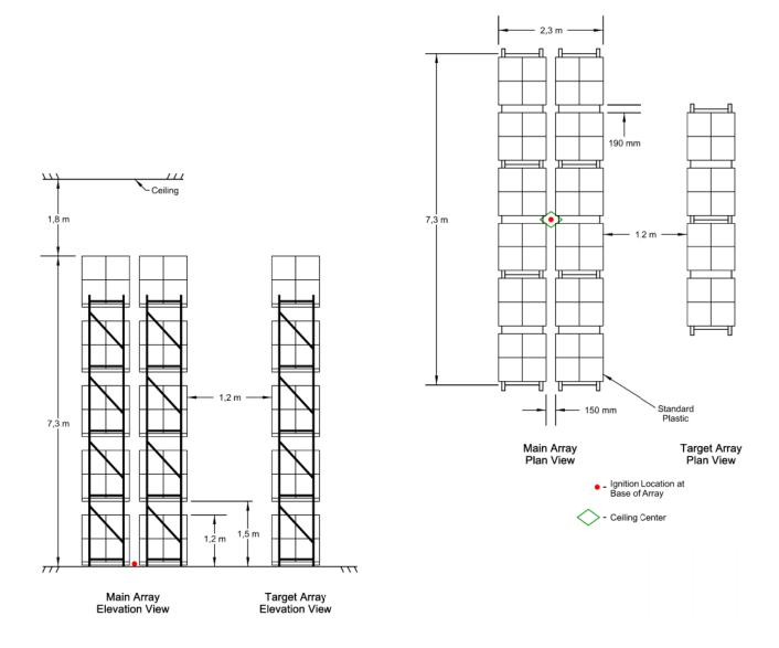
Figure A.1.3 Full scale fire test array for ESFR K202 upright, Test C
