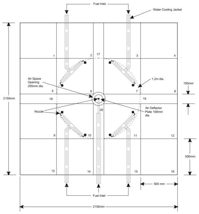
Non-flue pans are numbered 1-16. Flue pans are numbered 17-20.
