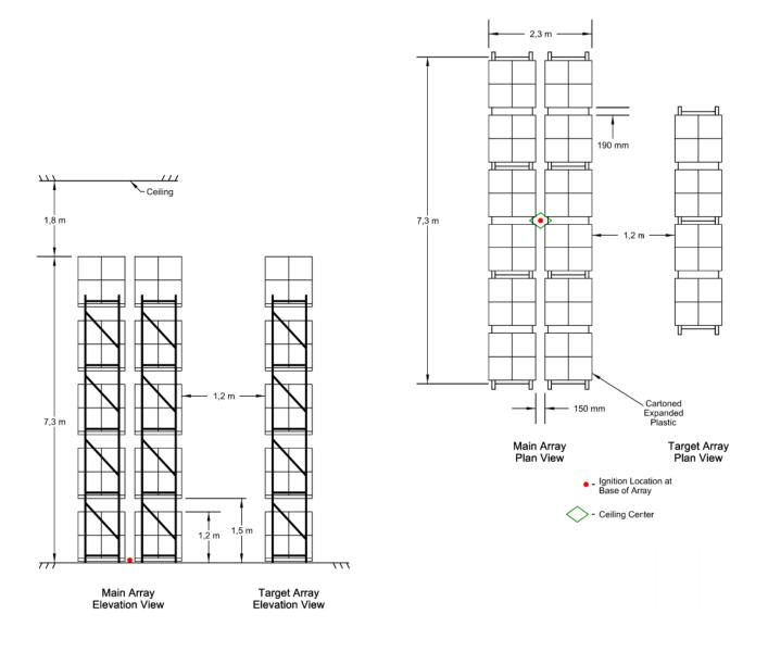
Figure A.2.2 Full scale fire test array for ESFR K240 upright, Test B
