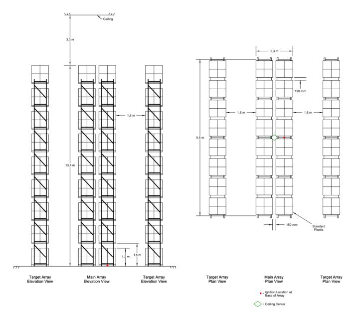
Figure A.5.2 Full scale fire test array for ESFR K480 pendent, Test B and C
