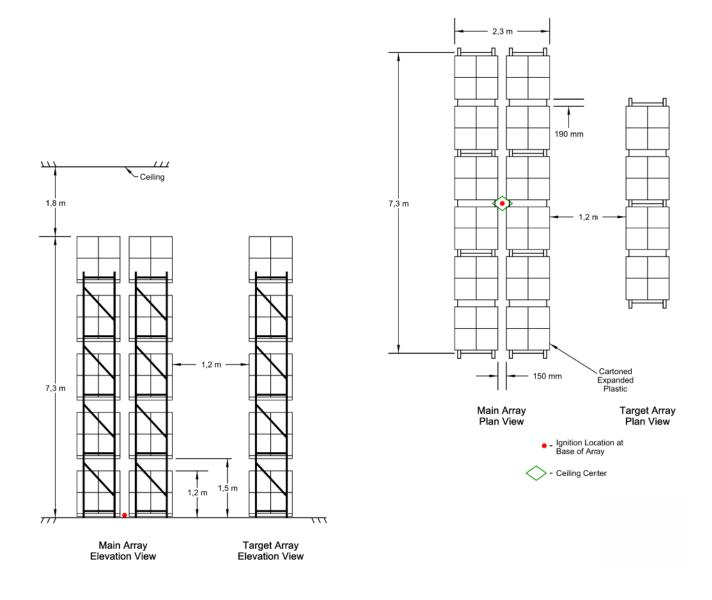
Figure A.1.2 Full scale fire test array for ESFR K202 upright, Test B
