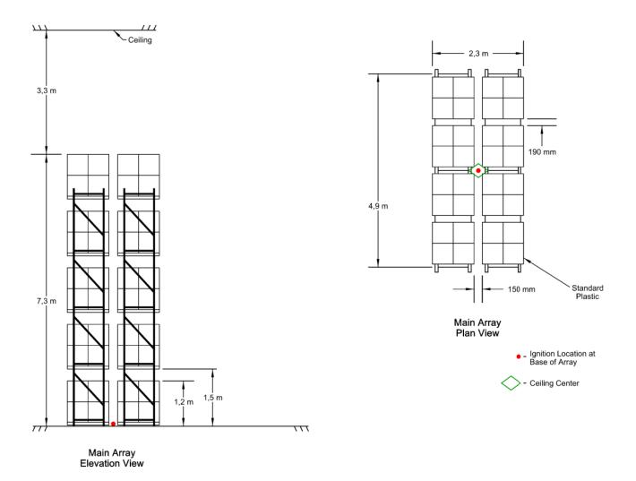
Figure A.2.4 Full scale fire test array for ESFR K240 upright, Test D
