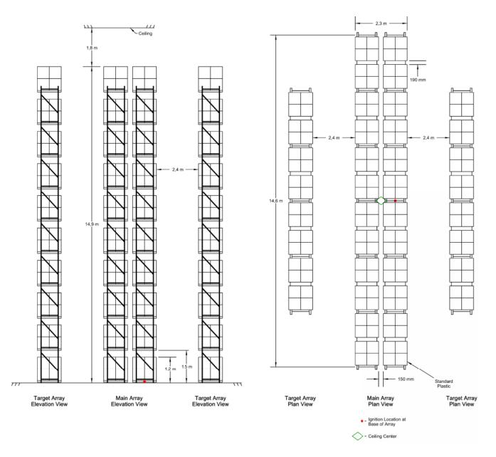
Figure A.4.1 Full scale fire test array for ESFR K400 pendent, Test A
