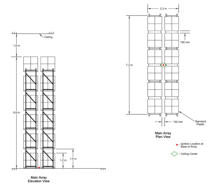
Figure A.2.5 Full scale fire test array for ESFR K240 upright, Test E
