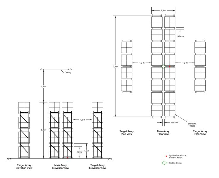
Figure A.6.2 Full scale fire test array for ESFR K202 and K240 pendent, Test B and C
