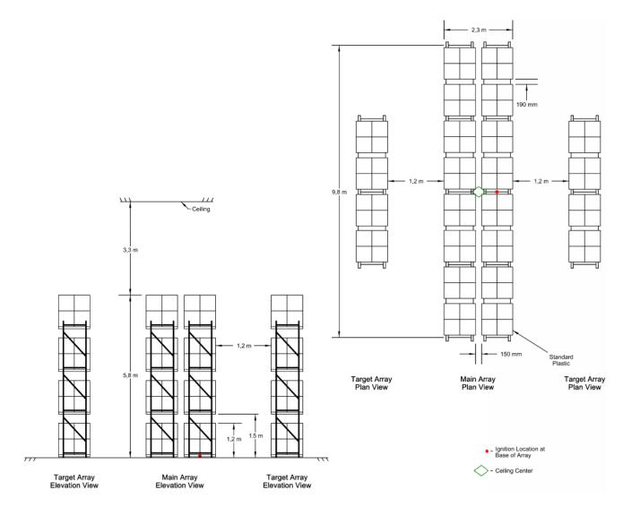
Figure A.3.2 Full scale fire test array for ESFR K325 and K360 pendent, Test B and C
