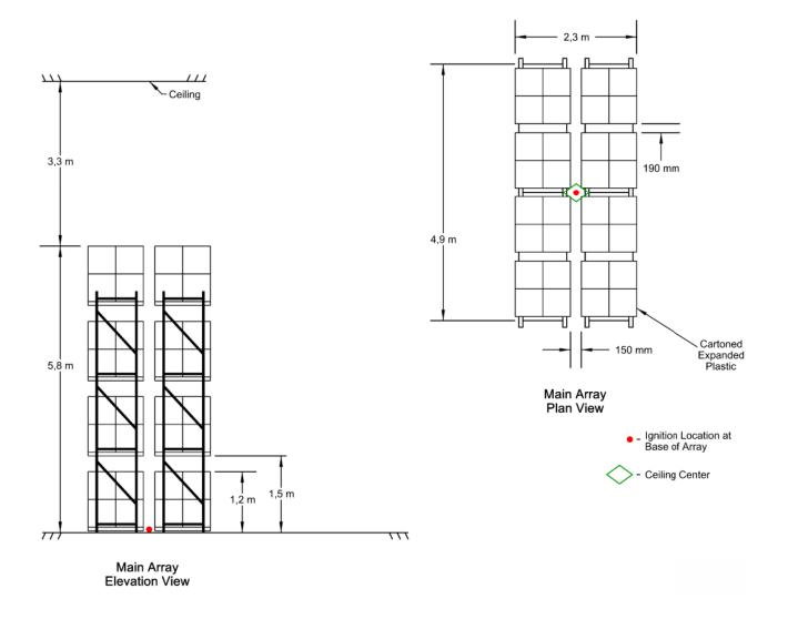
Figure A.1.1 Full scale fire test array for ESFR K202 upright, Test A
