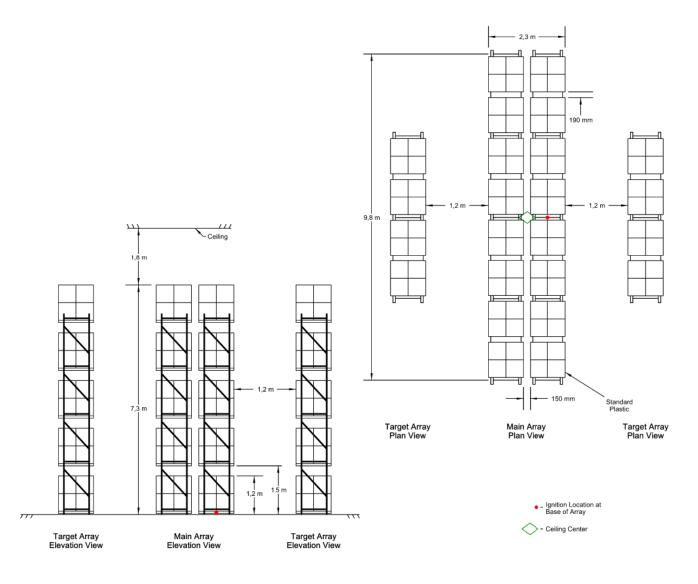
Figure A.3.1 Full scale fire test array for ESFR K325 and K360 pendent, Test A
