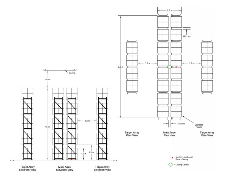
Figure A.6.1 Full scale fire test array for ESFR K202 and K240 pendent, Test A
