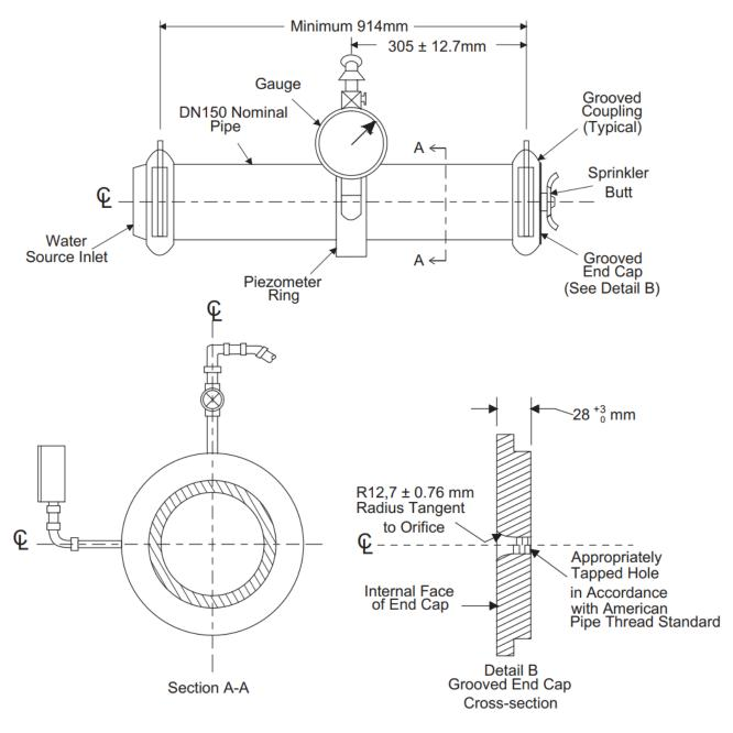
Note: All dimensions are nominal size unless otherwise indicated. Radius on Inlet may be truncated on internal face.
