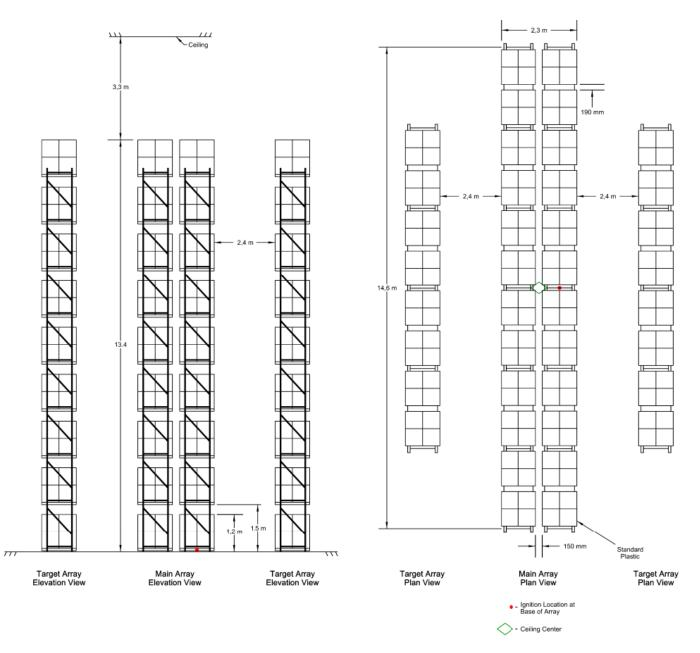
Figure A.4.2 Full scale fire test array for ESFR K400 pendent, Test B and C
