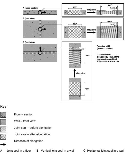
Figure 14 – Test condition with lateral elongation at the maximum of the nominal width
