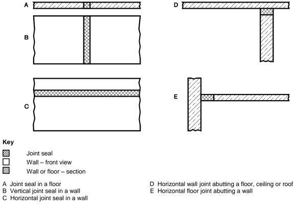
Figure 1 – Possible orientations of linear joint seals
