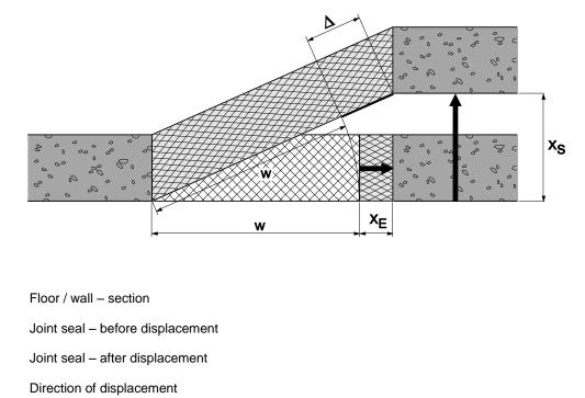
$\Delta$  Displacement equalling 100% of the movement capability given by the manufacturer
