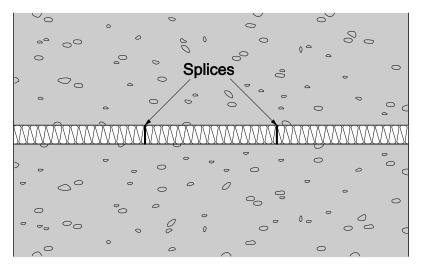
Figure 18 – Mineral wool – Distance between splices
