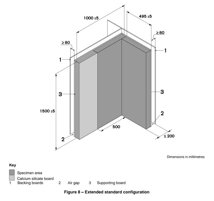
When using the configuration according to Figure 8 the part of the wing that is not covered by the test material shall be made of calcium silicate board.
