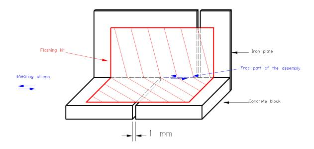
The system is the placed in a cold box set at a temperature of  $(-20 \pm 2)$  °C. The gap spacer is then removed and the system is subjected to 500 movement cycles in accordance to EOTA TR 008.
