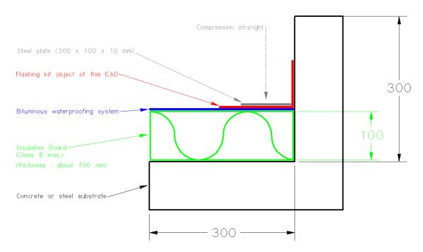
A charge of compression shall be applied with a steel plate (300 x 100 x 10 mm) until the ruin of the system (indicative value). Based on experience, the resistance to walking is given, if the measured values of compression strength for 10% relative deformation is over 60 kPa. Otherwise the resistance to walking cannot be verified on the basis of this EAD. Where relevant, a more exact test method for the resistance to walking of the kit would be need.
