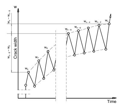
Figure F.4.3 Assessment of crack width stabilisation
