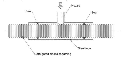
Figure 2.2.7.1 Tightness test – Schematic
