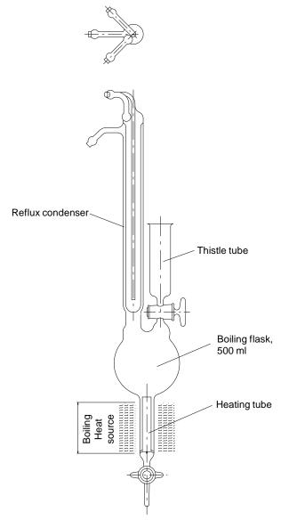
Figure G.1.1 Glass extraction apparatus
