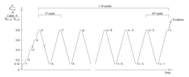
Figure F.2.1 Loading sequence in load transfer test
