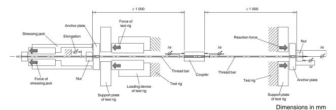
Figure D.2.1 Static load test – Schematic
