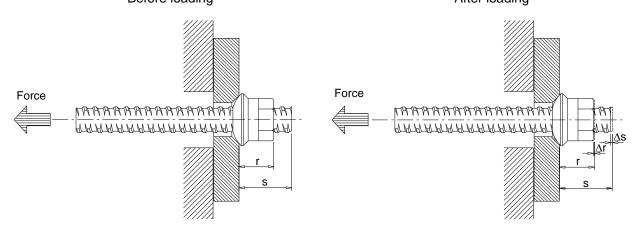
Figure D.4.1 Displacements during testing – Schematic example
