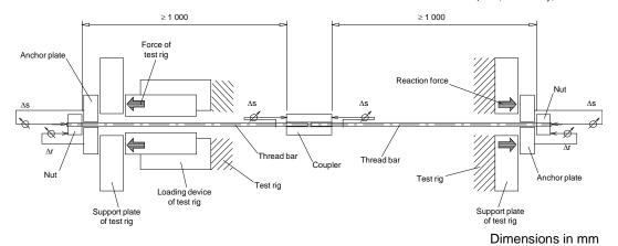
Figure E.2.1 Fatigue test – Schematic example with two anchorages and one coupling assembly
