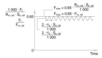
Figure E.2.2 Force in fatigue test – Schematic
