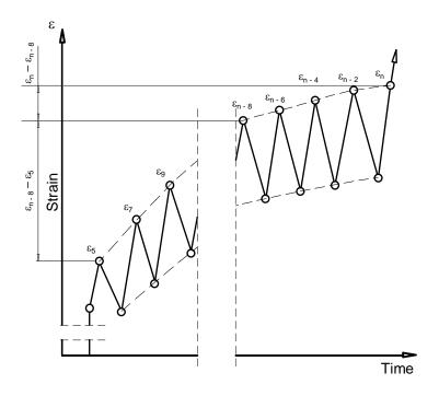
Figure F.4.4 Assessment of strain stabilisation
