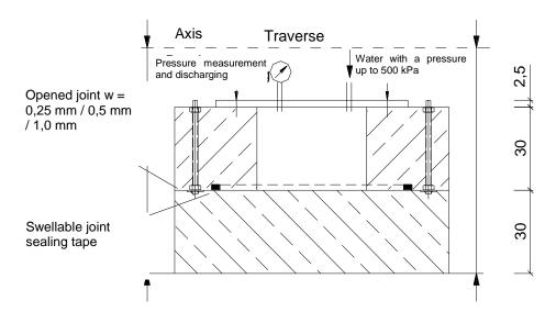
The two-part concrete test specimens shall be made of watertight concrete, e.g. the following composition:
