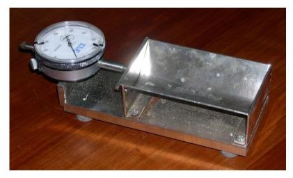
Figure B.5 - Extensometer
