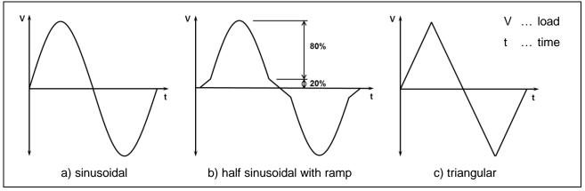
Figure E.9 Permitted seismic shear cycle C1.2
