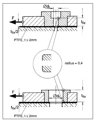
Figure D.6 Examples of shear test sleeves
