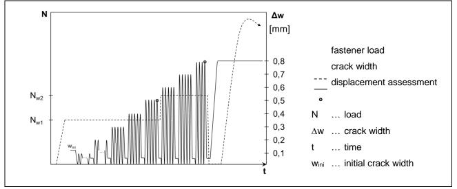
Figure E.13 Schematic test procedure C2.5
