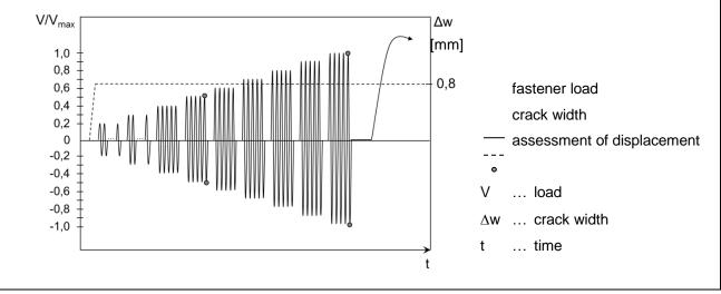
Figure E.11 Schematic test procedure C2.4
