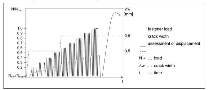
Figure E.10 Schematic test procedure C2.3
