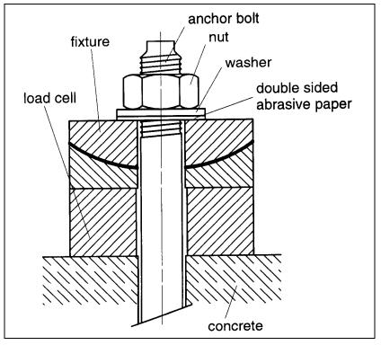
Figure D.8 Example for torque test (schematic)
