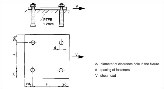
Figure D.13 Dimensions of fixture
