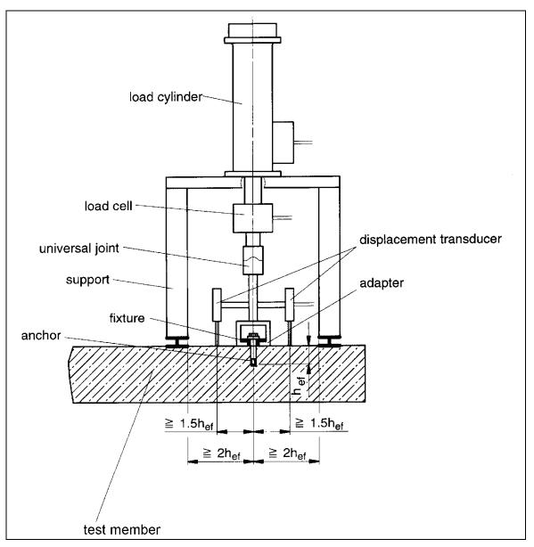
Figure D.3 Example of a tension test rig for <u>unconfined</u> tests
