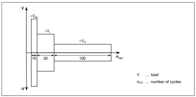
Figure E.8 Required load history for test series C1.2
