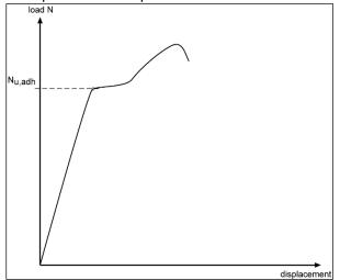
Figure A.2 Load at loss of adhesion by a significant change of stiffness
