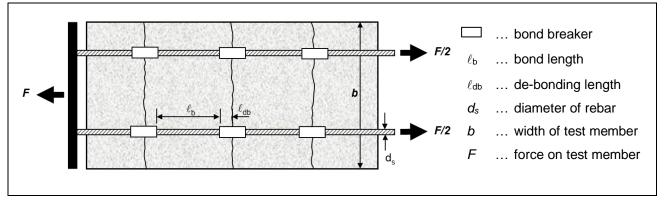
Figure E.2 Example for test member with bond breaking pipes on rebar (plan view)
