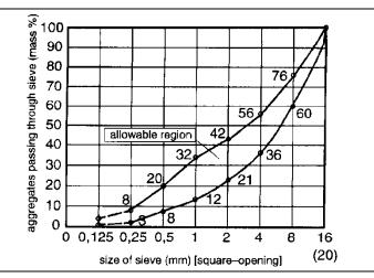
Figure D.1 Admissible region for the grading curve
