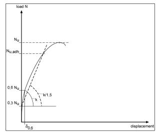
Figure A.5 Evaluation of load at loss of adhesion
