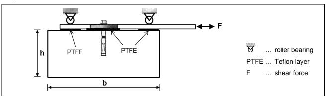
Figure E.5 Sketch of example for shear test setup with no significant friction forces
