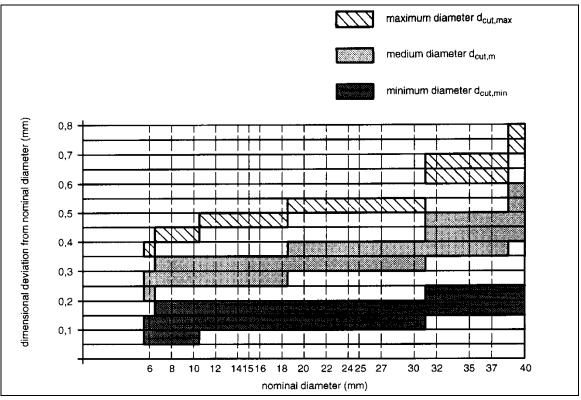
Figure D.5 Cutting diameter of hard metal hammer-drill bits
