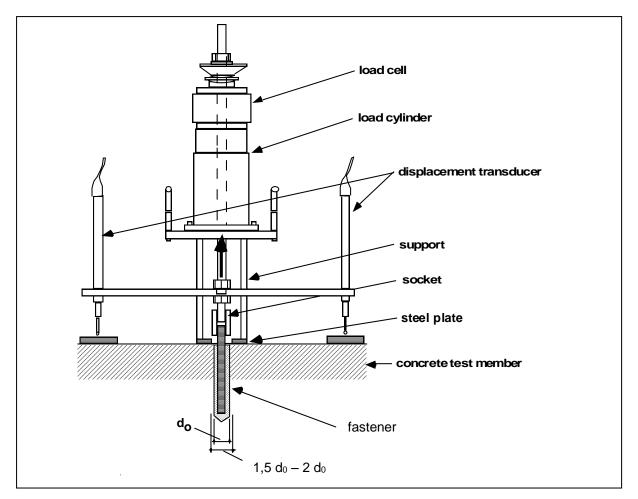
Figure D.4 Example of a tension test rig for <u>confined</u> tests
