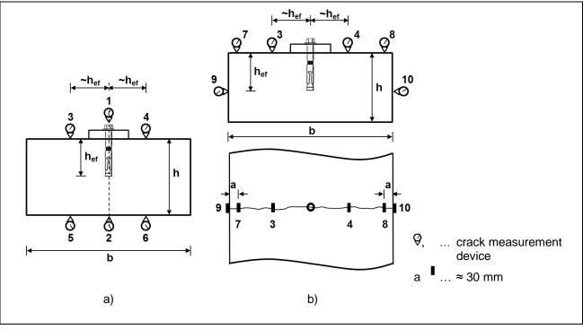
Figure E.3 Measurements to show fulfilment of the constant crack width requirement
