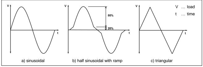
Figure E.12 Permitted seismic shear cycle C2.4
