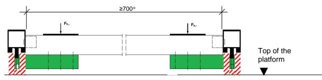
\*dimensions according to the H test samples in EN 16758
