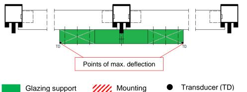
Figure B.3 Exemplary presentation of test setup and position of the load (cruciform glazing support, double-sided)
