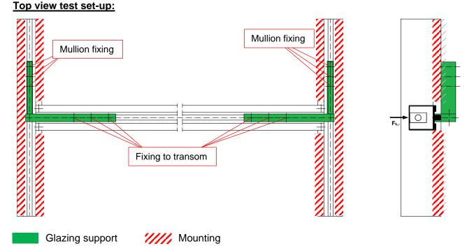
Figure B.5 Test setup and position of the load (wind suction)
