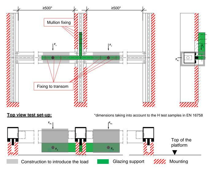
Figure B.7 Test setup and applied load direction (cruciform glazing support, double-sided combined load)
