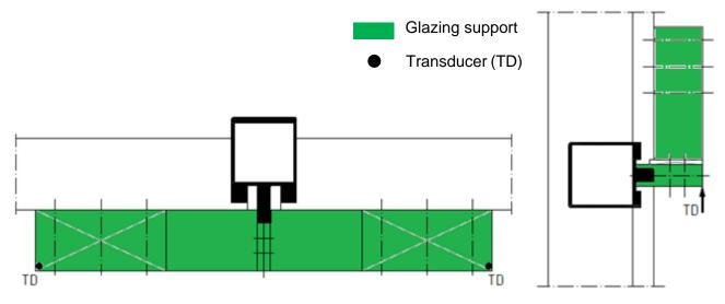
Figure B.2 Position of the transducers
