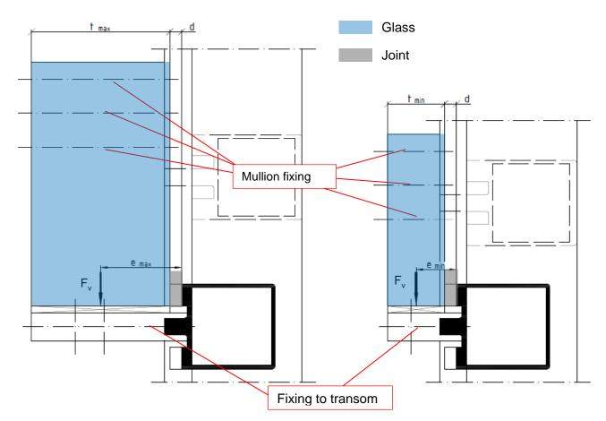
Figure B.1 Eccentricities for minimum and maximum glass thickness (cruciform glazing support)
