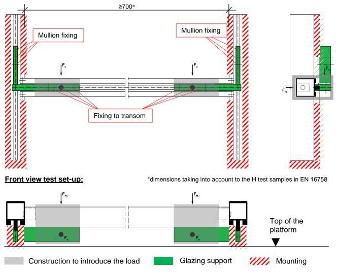
Figure B.8 Test setup and applied load directions (cruciform glazing support, one-sided combined loads)
