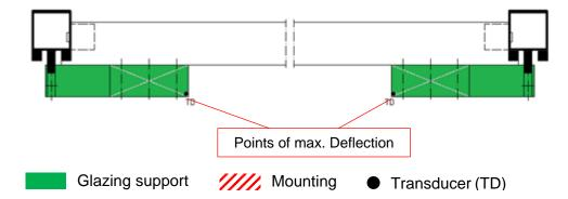
Figure B.4 Exemplary presentation of test setup and position of the load (cruciform glazing support, one-sided)
