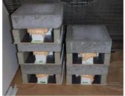
Figure F.5 Test sample during curing (48hrs)
