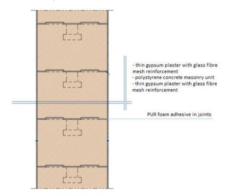
Example vertical section of an assembled internal wall
