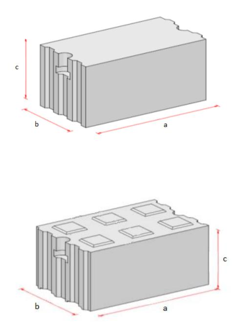
Example shapes of polystyrene concrete masonry units
