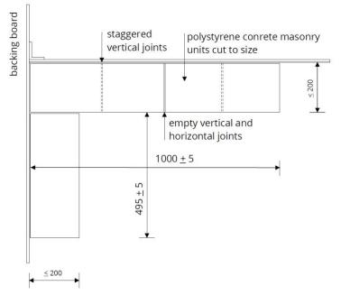
Figure D.1 Test rig configuration for polystyrene concrete masonry units
