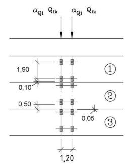
The numbers 1, 2 and 3 correspond to the lane numbers *Figure D.4: Tandem system arrangement*
