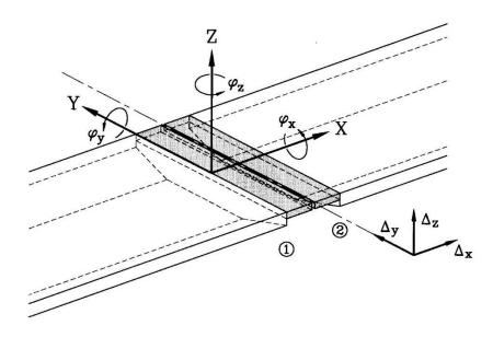
Figure D.7: Combination of movements
