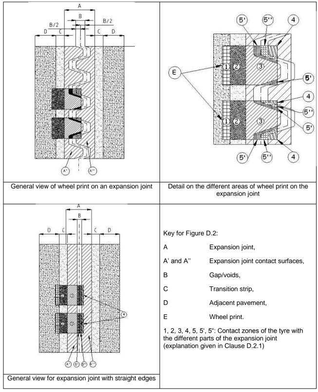
Figure D.2: Principles of wheel load distribution
