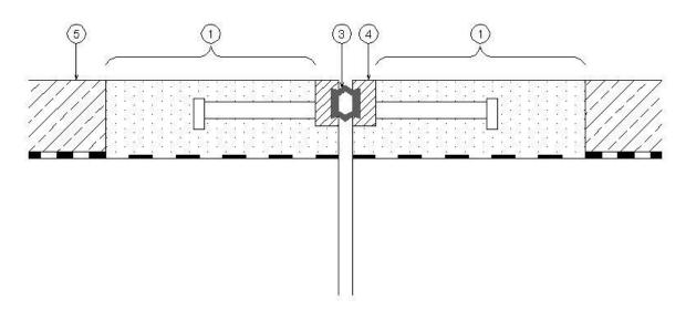
d) A combination of adhesion to the bridge deck concrete completed by fastening of reinforcement into holes
