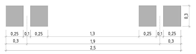
Figure D.3: Wheel print (dimensions are in m)
