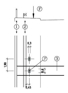
Key: ① Pedestrian parapet ② Safety barrier ③ Expansion joint  $F = A_d/2 = 100 \text{ kN}$
