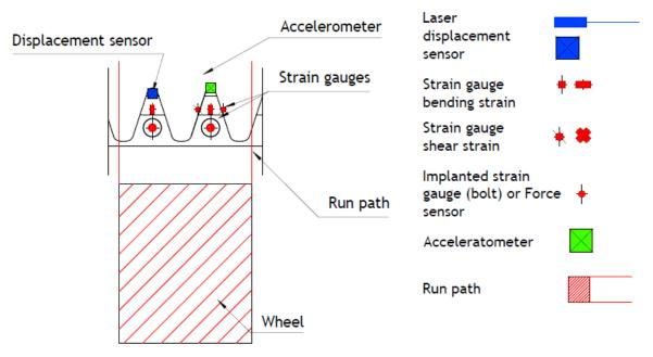
Figure C.2: Transverse position for over rolling
