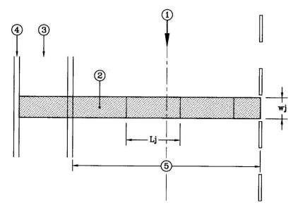
Key: ① Traffic direction ② Expansion joint ③ Footpath ④ Pedestrian parapet ⑤ Lane
