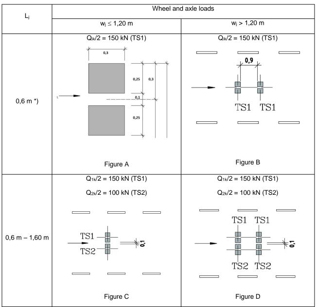
Table D.2: Wheel and axle loads (dimensions are given in m) Key: → Traffic direction
