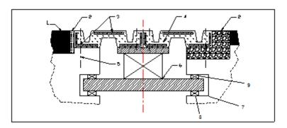
Figure 4: Example for supported multiple mat expansion joints
