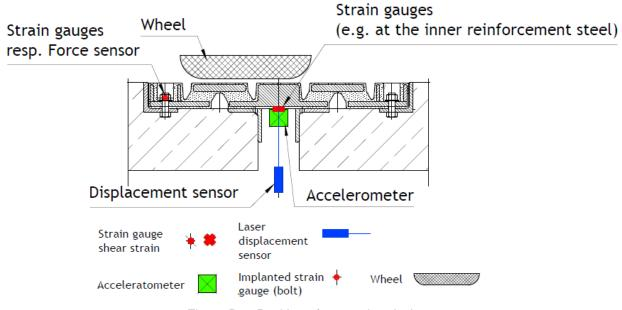
Figure D.1: Position of measuring devices
