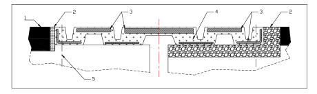
Figure 1b: Example for multiple Mat Expansion Joints on the basis of shear deformation
