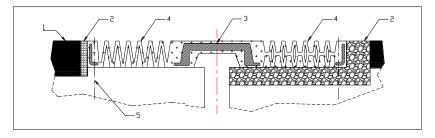
Figure 3: Example for single Mat Expansion Joints on the basis of compression/tension deformation including reinforcement/bridging plate
