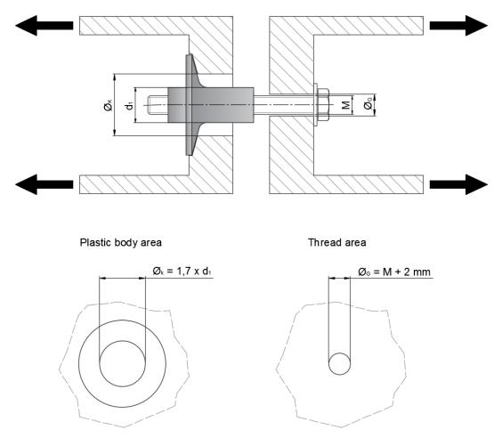
Figure A.1: Test rig for tension tests (sectional view) with bearing plates at both ends
