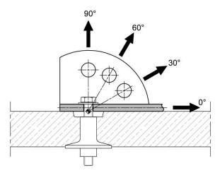
Figure A.3: Examples of attaching points
