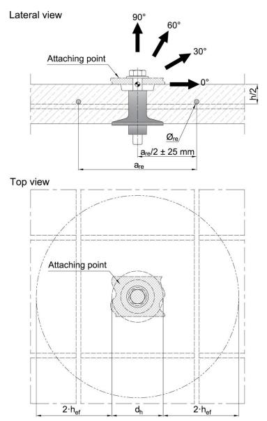
Figure A.2: Setup for tests in concrete
