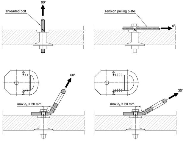
$\mathbf{e}_h$  : distance between fastener axis and curvature of the test fixture
