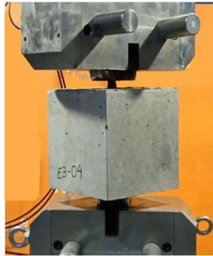
Figure A.2.1.1: Test setup for clamping kits that consist of three metallic pieces.
