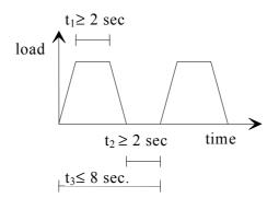
Figure 2 add 1 - Stress cycle for fatigue test with " $t_1$ " : duration of the peak load, " $t_2$ " : rest time,"  $t_3$ " total time of the cycle
