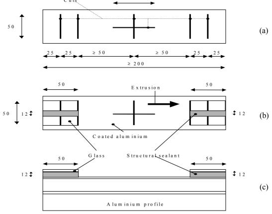
Fig. 1 add 1 - Sample for filiform corrosion tests
