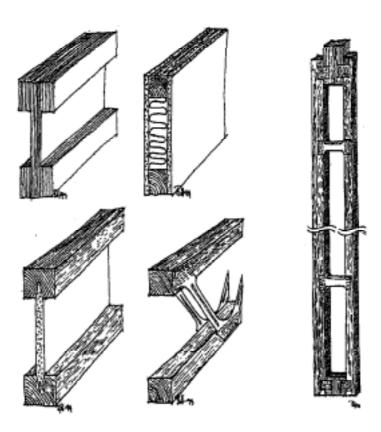
Figure 2.1. shows examples of light composite wood-based beams and columns used in building construction as structural members. Beams are primarily subjected to bending, shear and concentrated loads at the supports. Columns are primarily subjected to compressive forces in the axial direction, but also to transversal forces.
