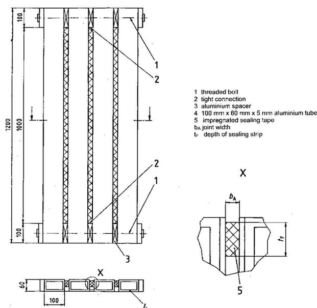
**Figure 2: Assembly for testing resistance to temperature fluctuations**
