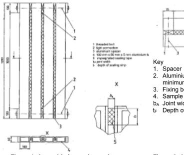
Figure 1: Assembly for testing resistance to temperature fluctuations
