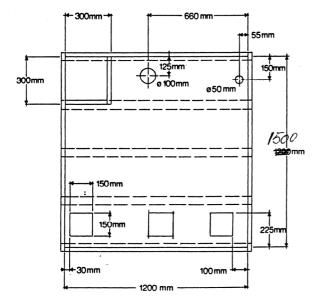
Figure 2. Plane view of test box
