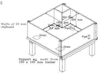
Fig. 1. Dimensions of the test floor.
