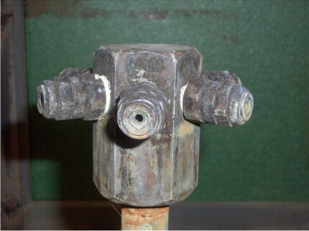
*Figure 4. Nozzles for water spraying.*
