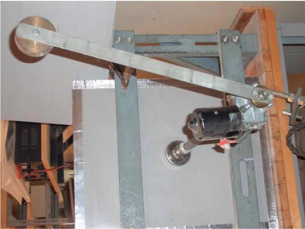
*Figure 5. Device for testing of bushings to dynamic load **Note: the photo is of an earlier device giving a more harsh load.***
