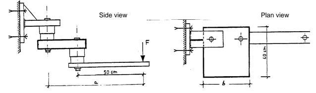
Figure E4. Examples of shear test equipment.
