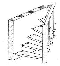
Figure B6: Stair with effective load-carrying barrier
