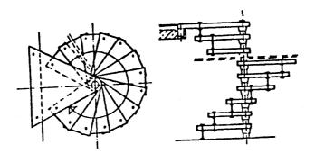
Figure B5: Spiral stair with loadbearing bolts
