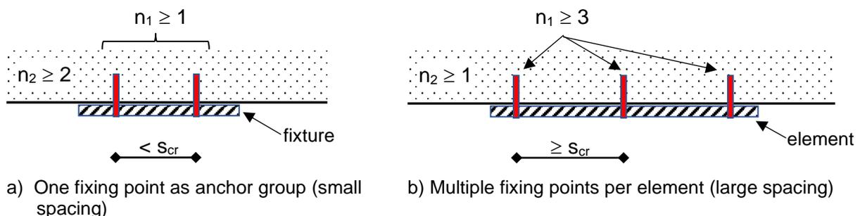
Figure 1.1: Examples of multiple injection anchor systems
