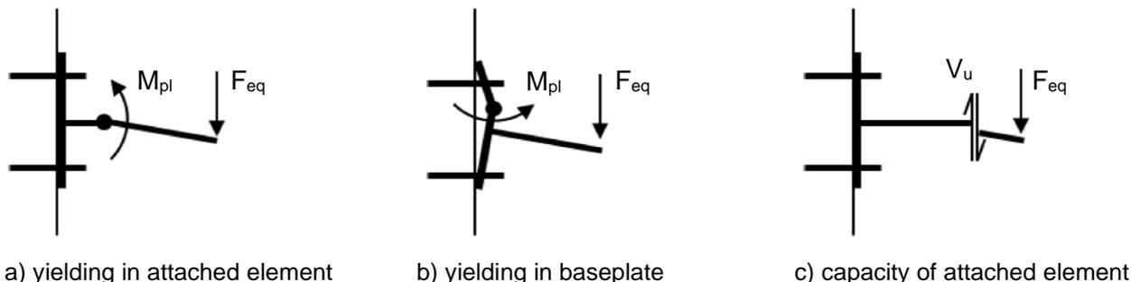
**Figure 6.1: Seismic design by protection of the fastening**
