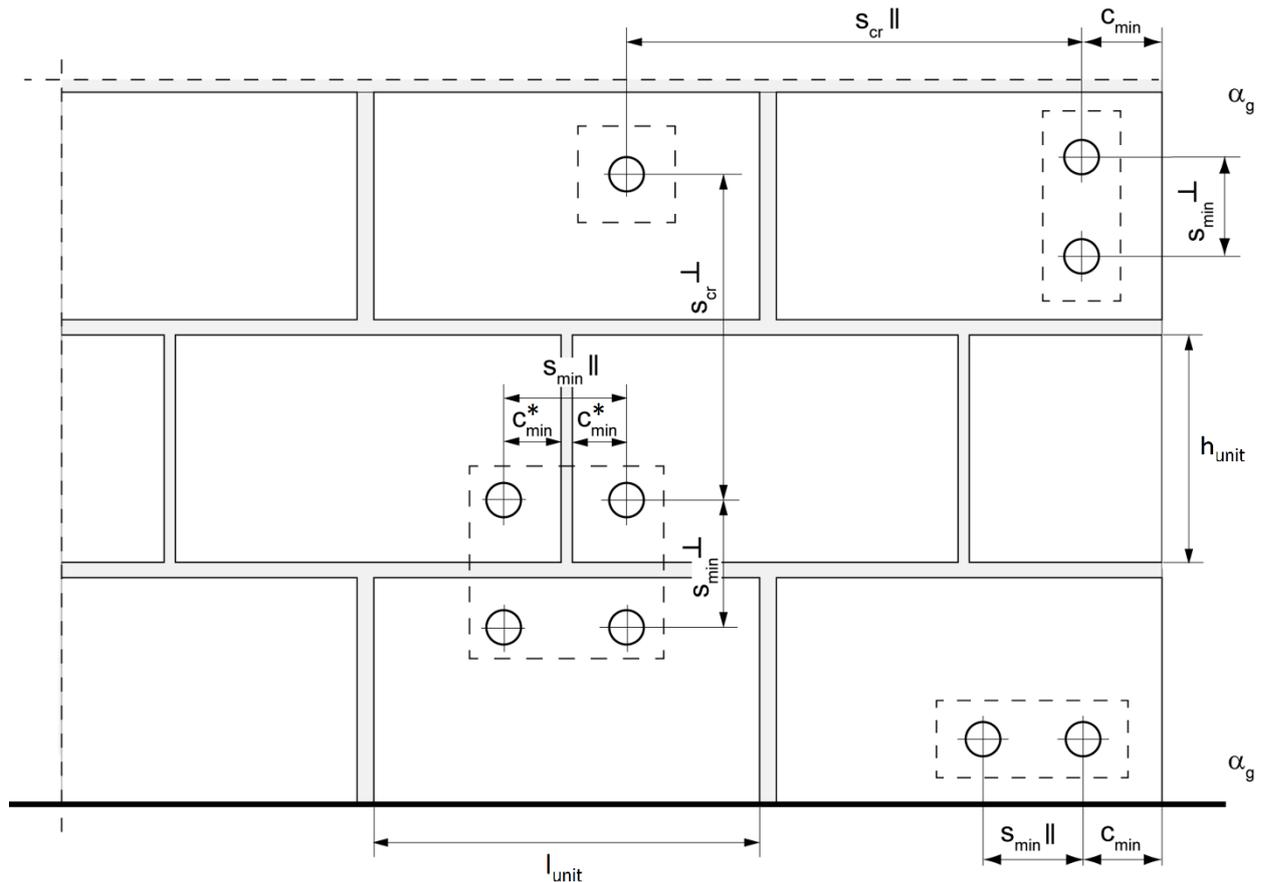
$c_{min}^*$  = minimum edge distance, only if vertical joints are not filled with mortar
