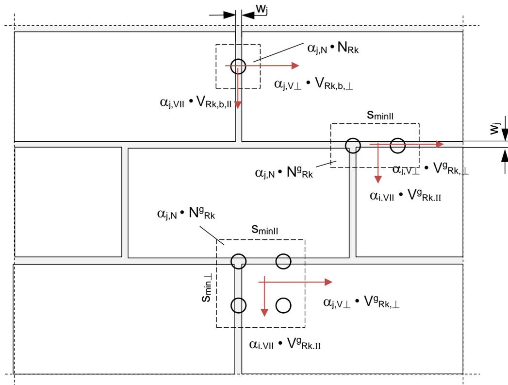
Figure 1.4: Reduction factors for resistances of screws in or near joints
