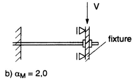
Figure 3.2: Fixture without (a) and with (b) restraint
