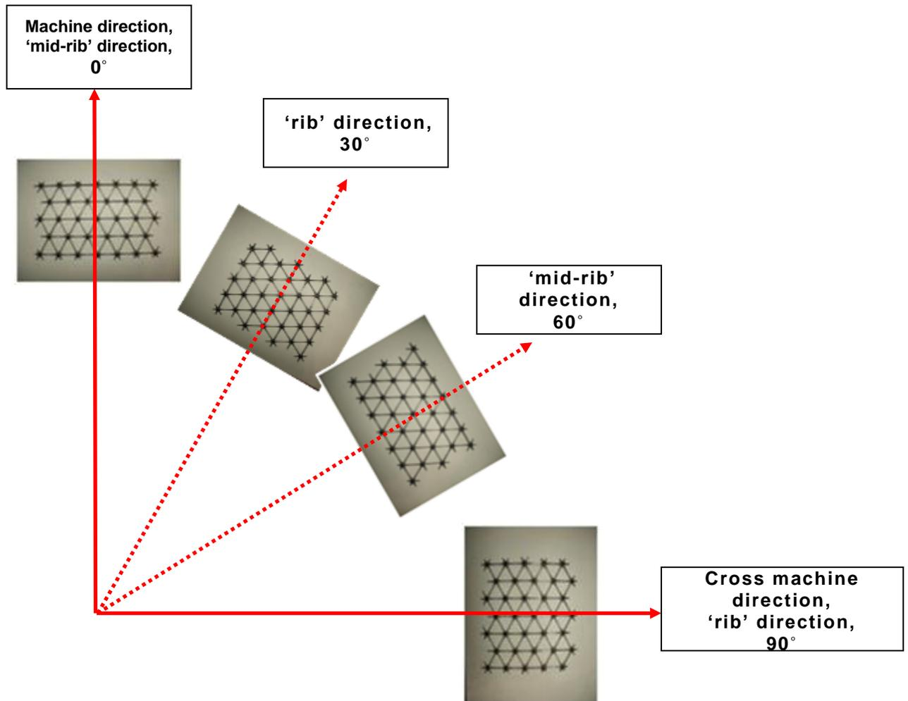
Figure 2- Schematic of testing directions
