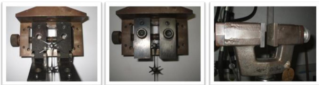
Figure 6- typical example of 'Junction strength' test clamps (6a & 6b show the upper junction clamp in open and closed positions; 6c shows the lower node/junction clamp)
