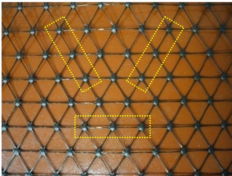
Figure 7 – Typical test specimen directions, four specimens required in each direction
