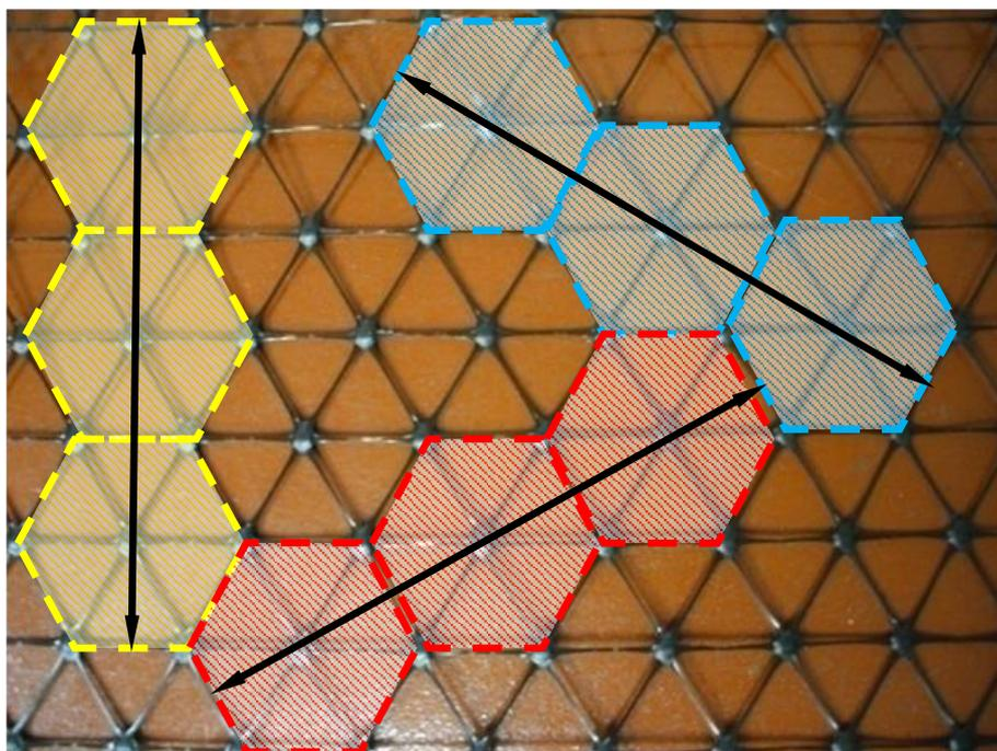
Figure 10- Three directions of measurement for hexagon pitch,
