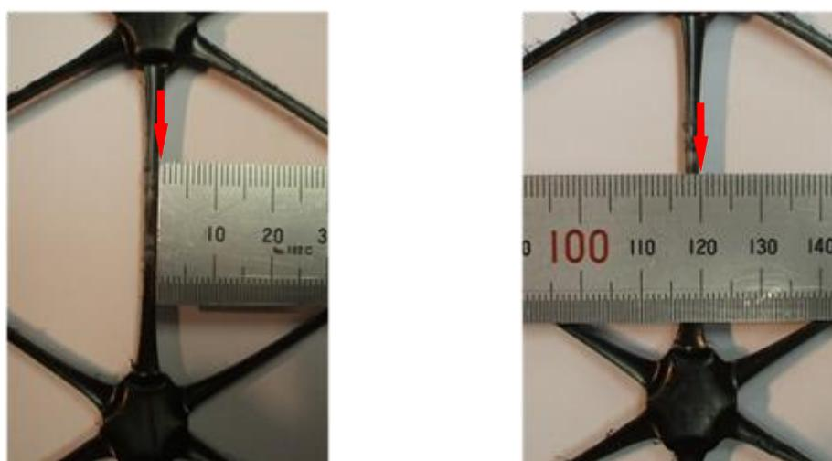
Figure 11 – Alignment of ruler during measurement
