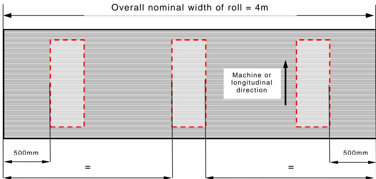
Figure 9- Measurement positions for hexagon pitch across the width of the role
