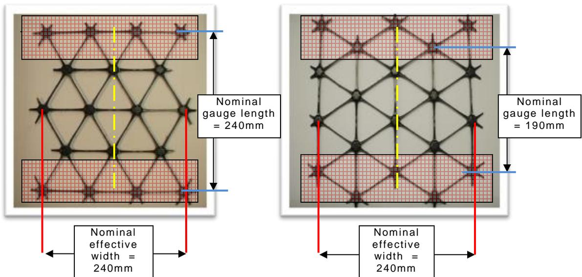
Figure 3.2 – example series nominal 120mm A/F repeating hexagon
