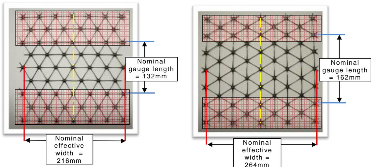
Figure 3.3 – example series nominal 66mm A/F repeating hexagon
