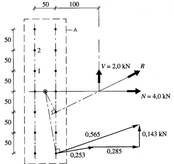
**Figure 8 - Nail connection subjected to an eccentric force.**
