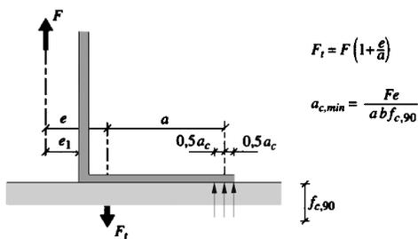
**Figure 4 - Angle bracket subjected to a lifting force.**
