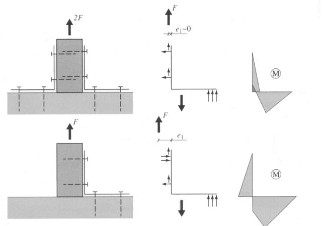
**Figure 5 - Connection with double and single angle brackets.**
