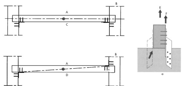
**Figure 2 - Anchoring of a purlin by means of purlin anchors and nails**
