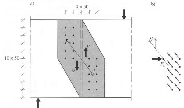
**Figure 9 - Connection with a fish-plate on each side.**
